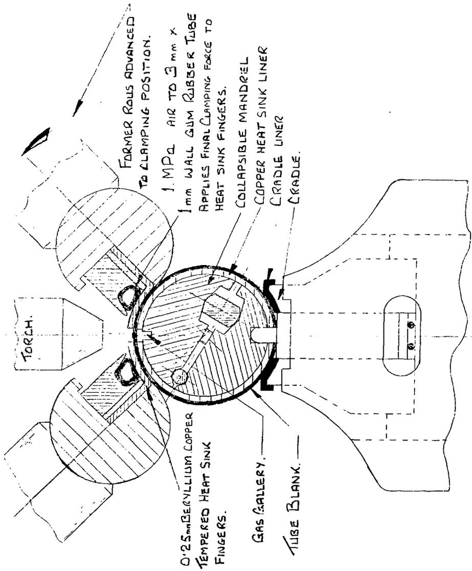
FIGURE 10 : CROSS SECTION OF FINAL ROLLING AND WELDING MACHINE
