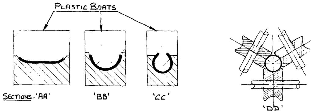
FIGURE 4 : SCHEMATIC OF THE GERMAN MILL TUBE WELDING MACHINE
