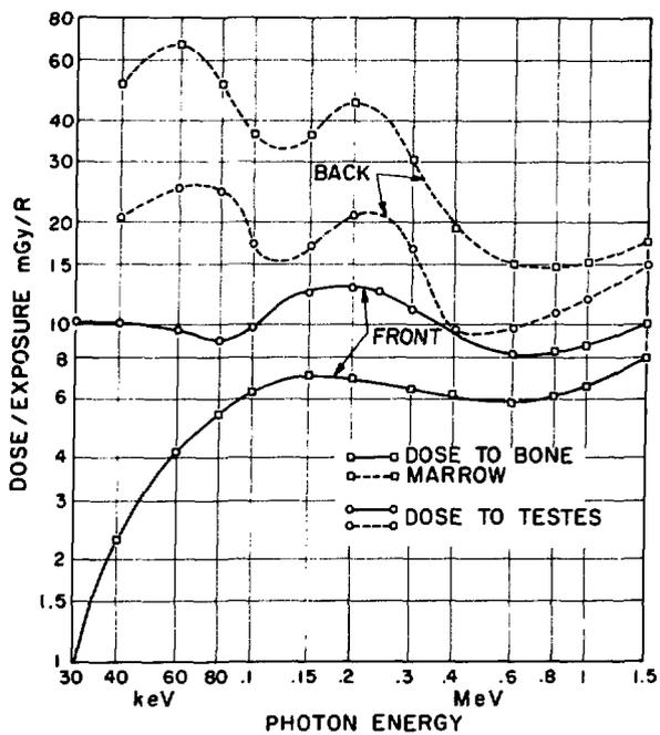
FIGURE 3. DOSE ABSORBED IN BONE MARROW AND TESTES PER EXPOSURE TO PERSONAL DOSIMETER
