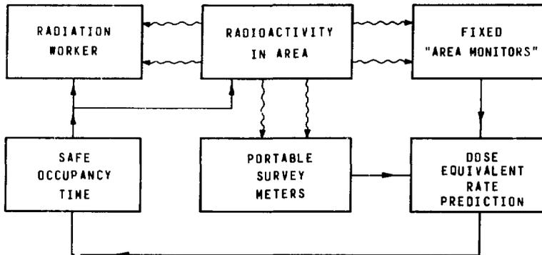
FIGURE 6. AREA MONITORING INSTRUMENTS
