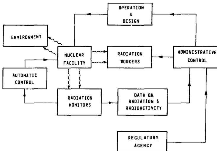
FIGURE 1. ROLE OF MONITORING INSTRUMENTS IN RADIATION PROTECTION
