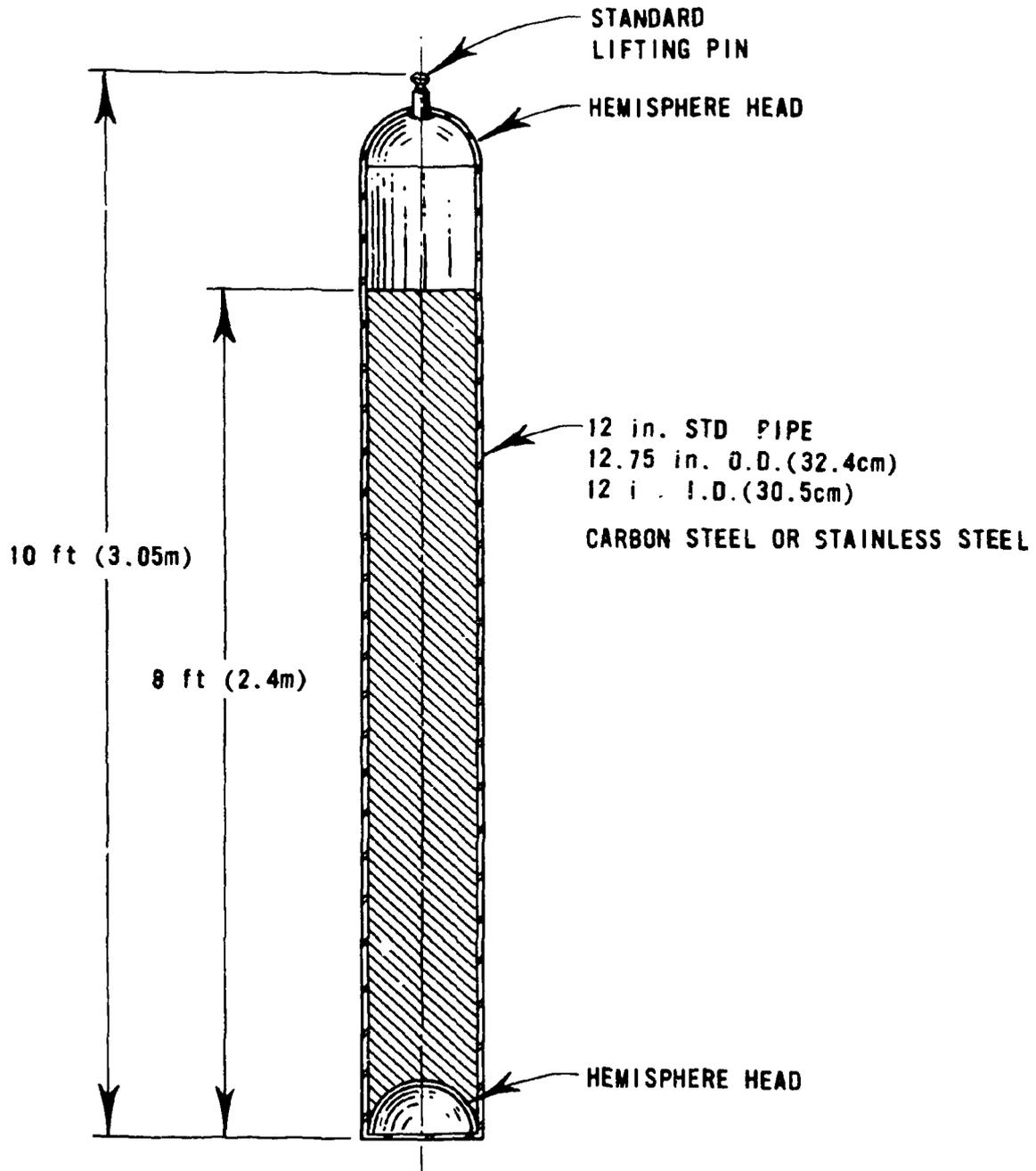
Fig. 2. Assumed standard canister for high-level, cladding, and intermediate-level wastes (generic repository description) (original figure: OWI-78-301).
