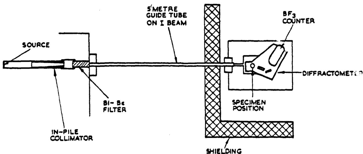
Fig. 3) Harwell guide tube and diffractometer for small-angle neutron scattering and diffraction from biological materials.
