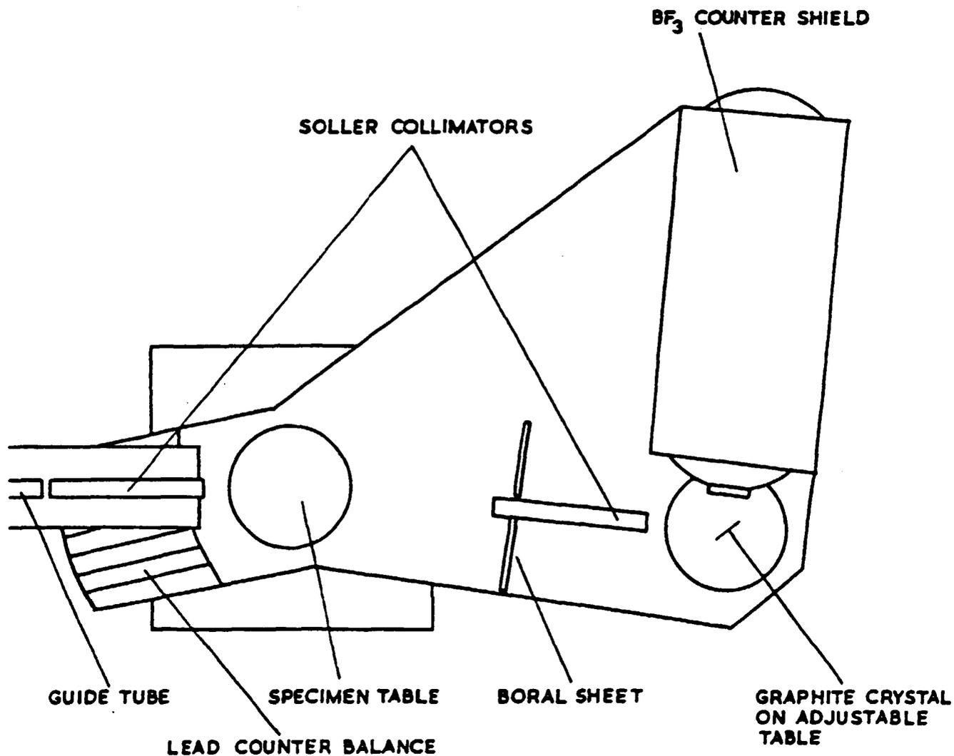
Fig. 4) Detail of diffractometer.
