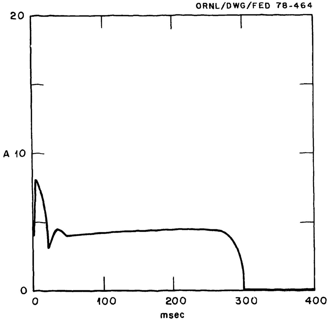
Fig. 3. Decel current waveform as displayed by VT-11 graphic terminal. Other waveforms which may be displayed are decel voltage, accel current, accel voltage, arc current, and beam current.
