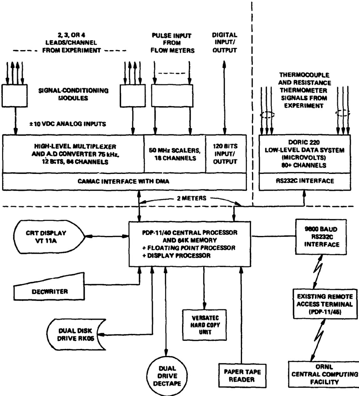
Fig. 1. Block diagram of the interactive data acquisition system for neutral beam development.
