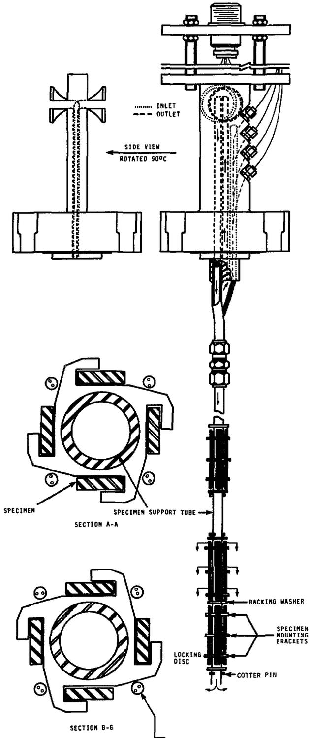
FIGURE 8: SCHEMATIC OF SAMPLE SUPPORT ASSEMBLY.
