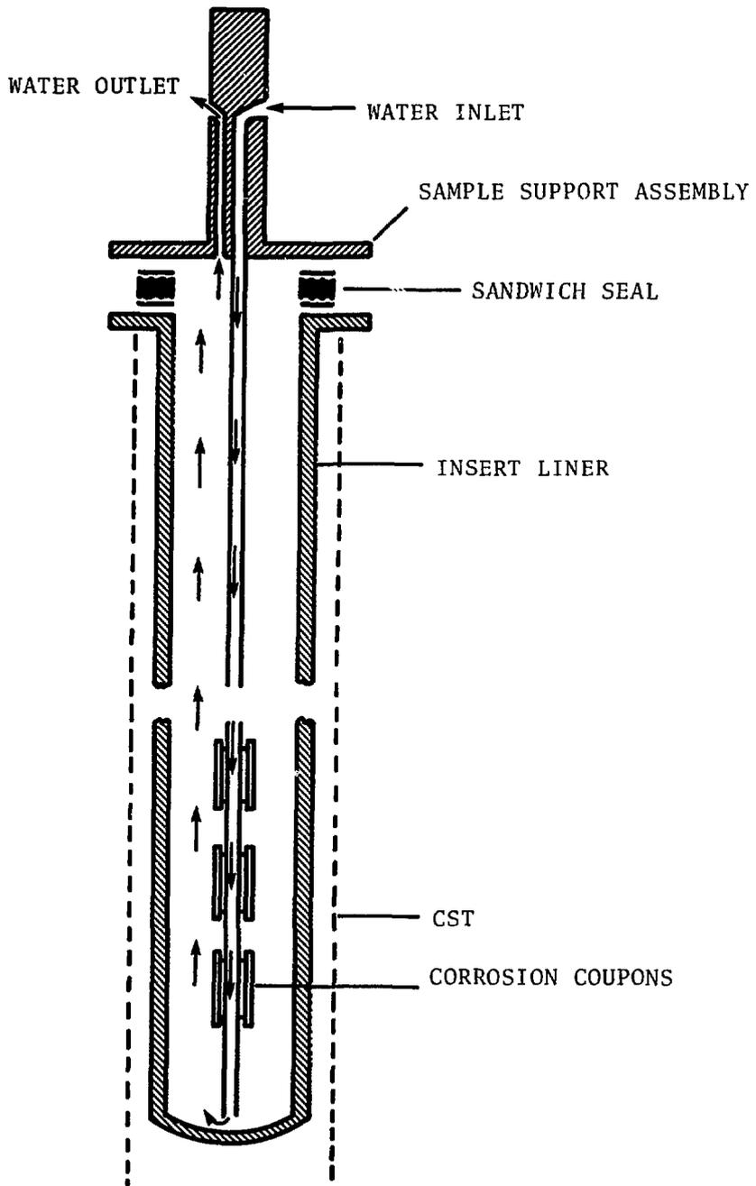
FIGURE 4: SCHEMATIC OF CORROSION TEST INSERT.
