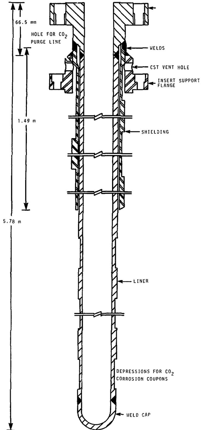
FIGURE 5: CROSS SECTION OF INSERT LINER
