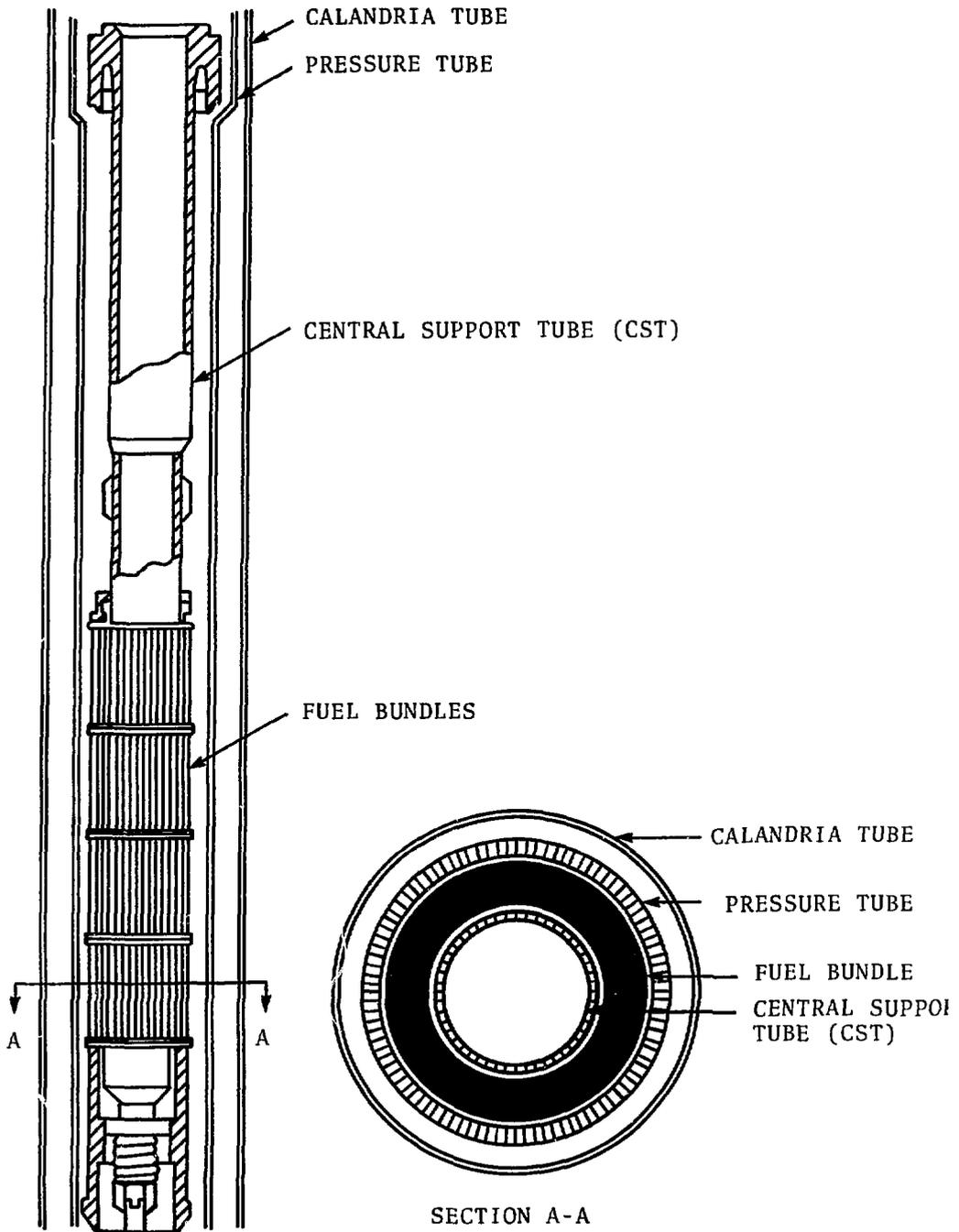
FIGURE 2: FUELLED PRESSURE TUBE.
