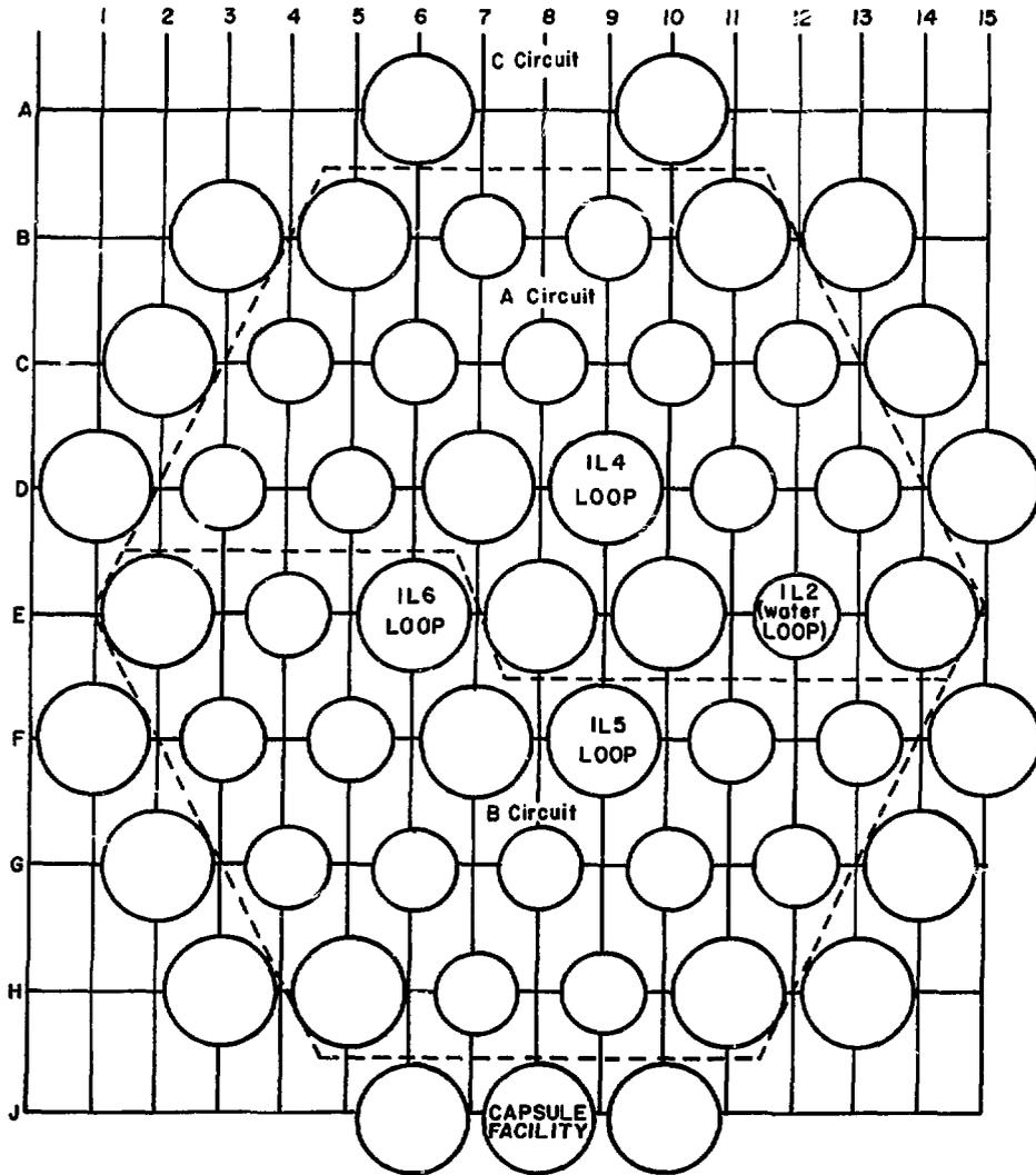
FIGURE 1: SCHEMATIC OF WR-1 REACTOR CORE LATTICE.
