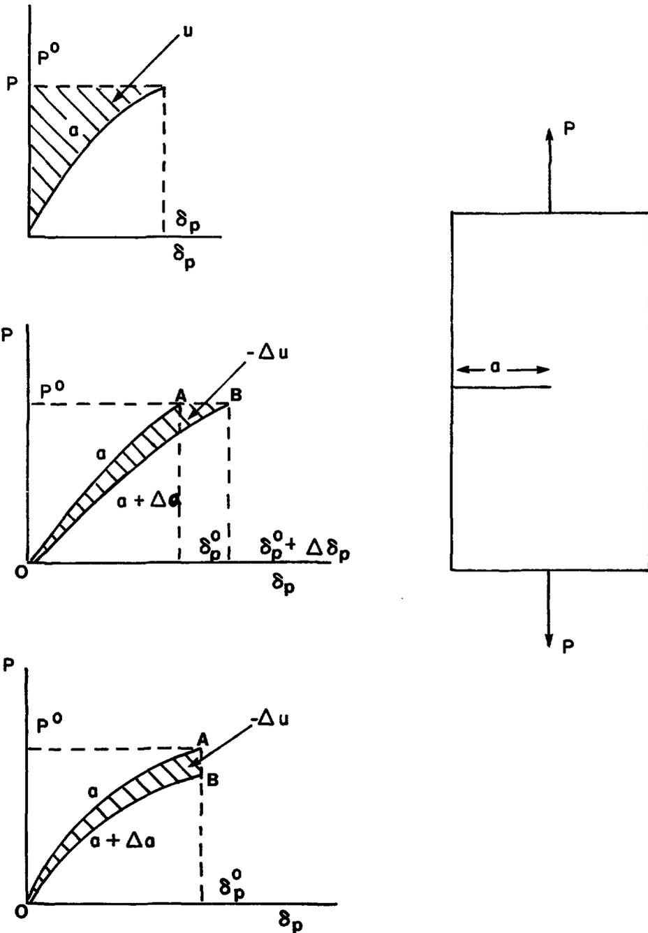
FIGURE 11: Load ( $P$ ) point deflection ( $\delta_p$ ) curves showing potential energy changes with crack extension (Reference 17)
