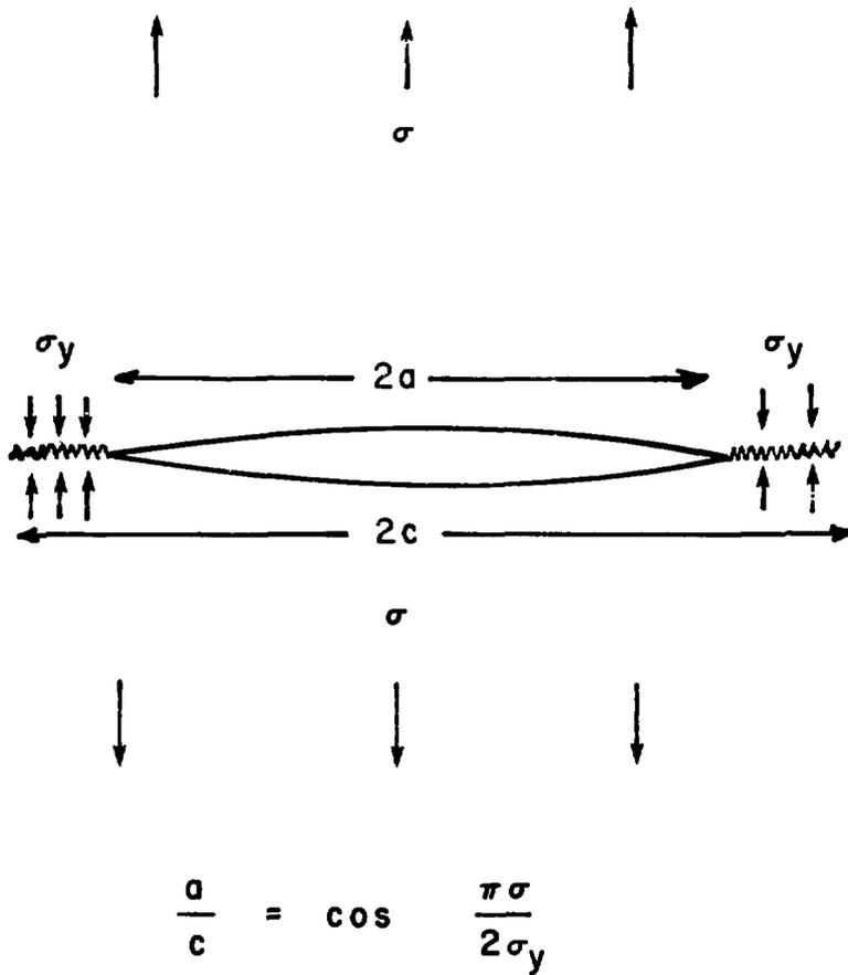
**FIGURE 4:** Dugdale model of "strip-yield" plastic zones under applied stress  $\sigma$ . Plastic zone size is  $c-a$ .
