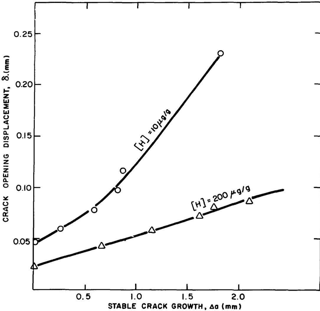
**FIGURE 9:** Application of the Smith and Knott method of determining  $\delta_i$  to Zr 2.5% Nb pressure tube material<sup>(13)</sup> (CT specimens).
