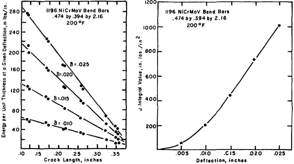
**FIGURE 14:** J-integral determination on steel by Begley and Landes<sup>(19)</sup>
