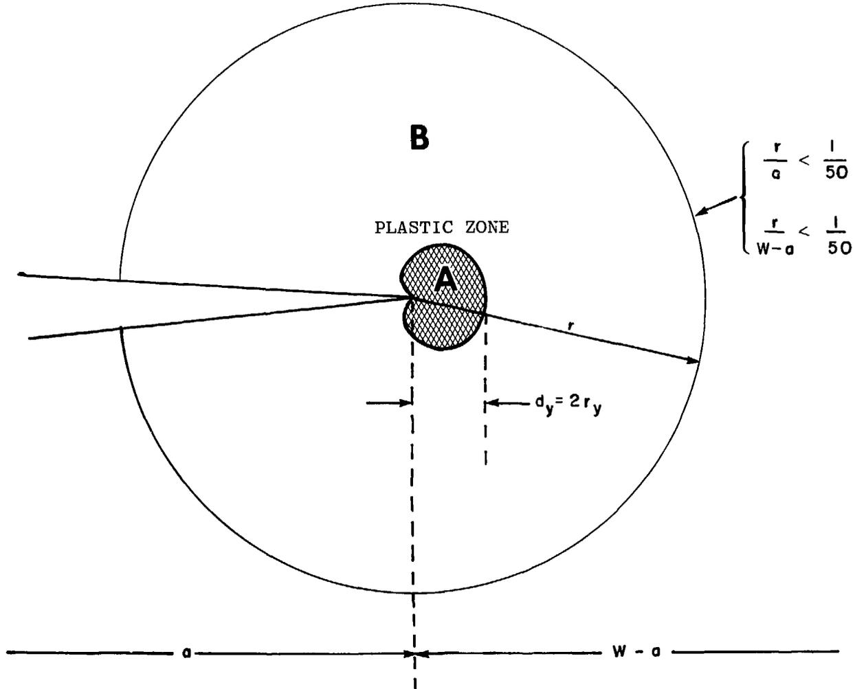
**FIGURE 3:** Crack tip region where  $K$  provides a one-parameter description of the stress field.  $a$ ,  $W$  as in Figure 1.
