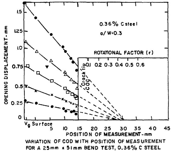
**FIGURE 8:** Method of calibrating clip gauge reading to give COD based on a fixed center of rotation
