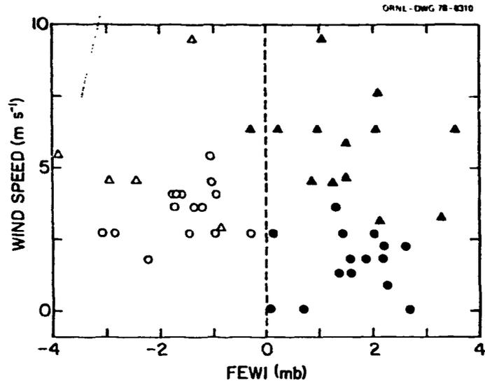
Fig. 4.2. Results of some recent tests of the ability of the Fog Excess Water Index to predict the formation of steam fog above heated water surfaces. Solid symbols indicate occasions in which fog was observed.
