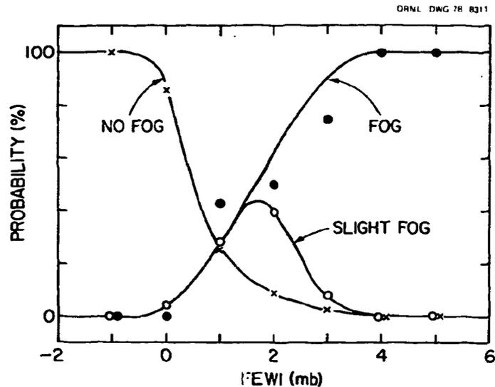
Fig. 4.3. The probability of finding fog, slight fog, or no fog above the Dresden, Illinois, cooling pond, based on meteorological data reported at Argonne.
