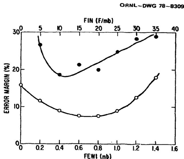
Fig. 4.1. A comparison of the Fog Index Number and the Fog Excess Water Index as indicators of the formation of steam fog. Data used are those of Currier et al.<sup>2</sup>
