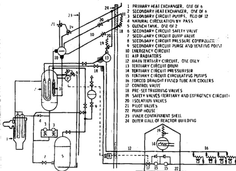
Figure A-1. Heat Disposal Circuit for the Dragon Reactor
