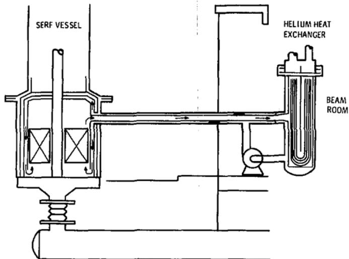
Figure G-5. HFFPR Helium Cooling Circuit
