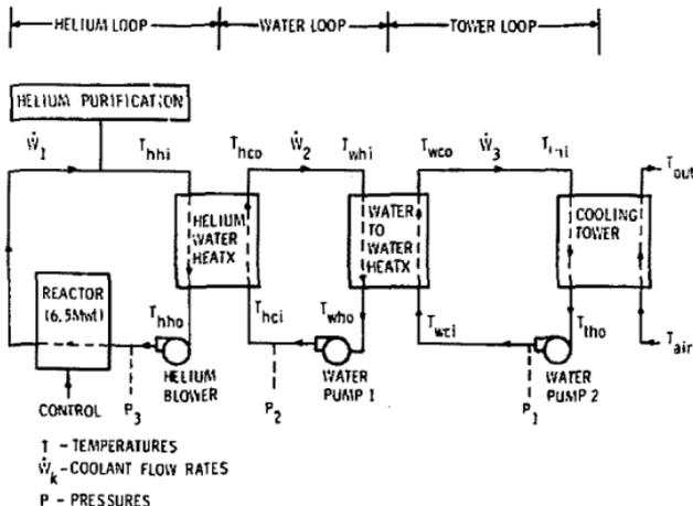
Figure B-1. Cooling System Block Diagram for HFFPP
