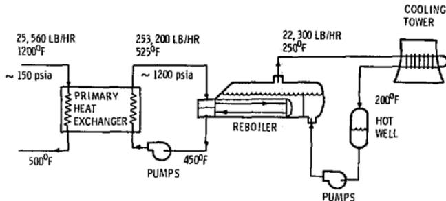
Figure C-3. Westinghouse Cooling System with Reboiler
