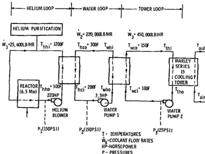
Figure C-4. HFFPR System Components and Nominal Design Conditions
