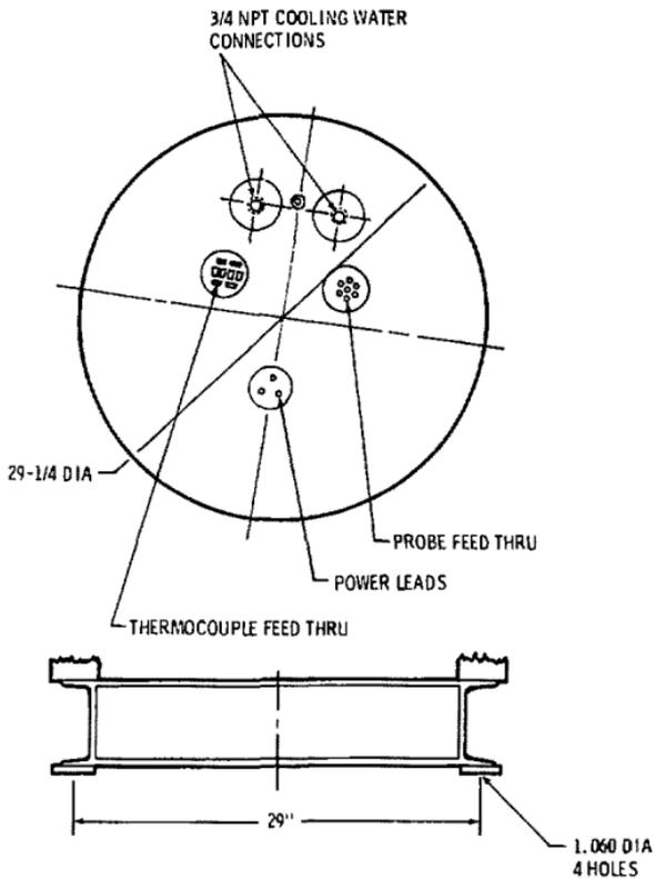
Figure D-3. Cross-Sectional Dimensions of the Helium Pump
