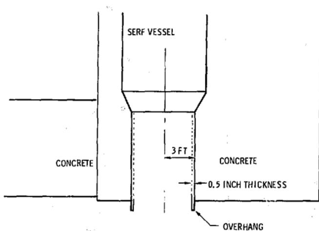
Figure F-1. Constraints on SERF Reactor Vessel
