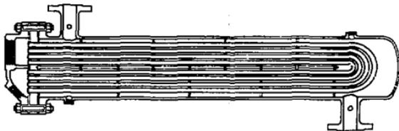
Figure C-1. U-Tube Heat Exchanger (Figure from Reference 11)
