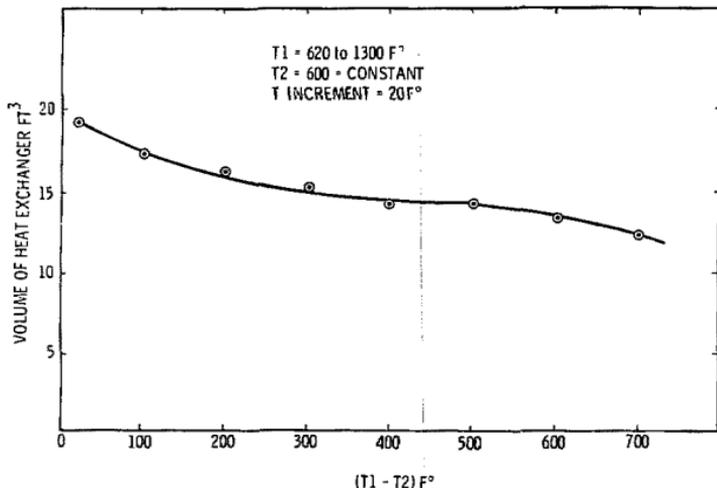
Figure H-2. Heat Exchanger Volume Variation with Temperature Increment
