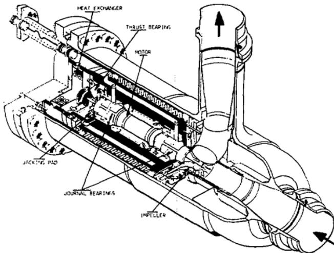
Figure D-1. Coolant Loop Blower
