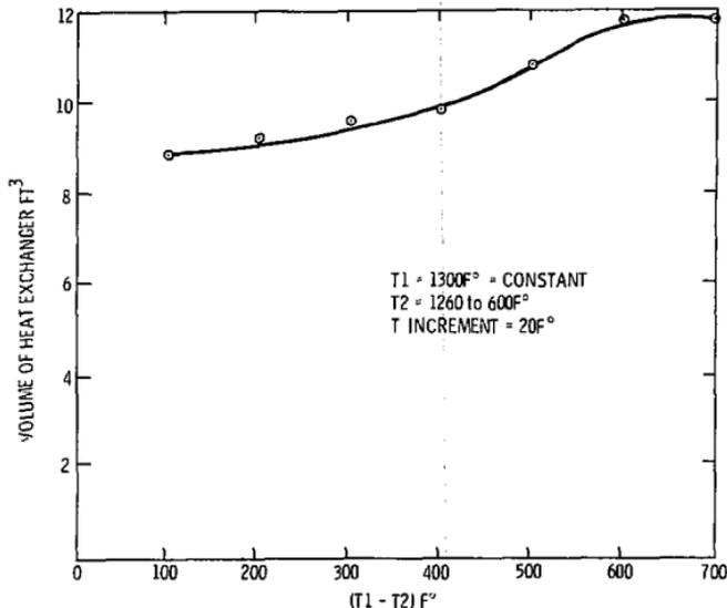
Figure II-1. Heat Exchanger Volume Variation with Temperature Increment
