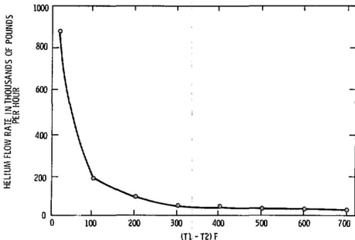
Figure H-3. Helium Flow Rate with Temperature Increment
