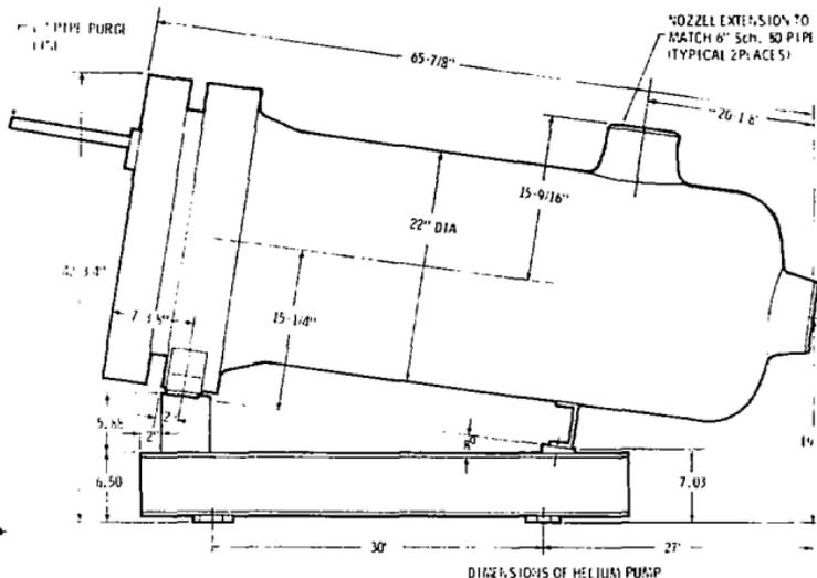
Figure D-2. Dimensions of Helium Pump
