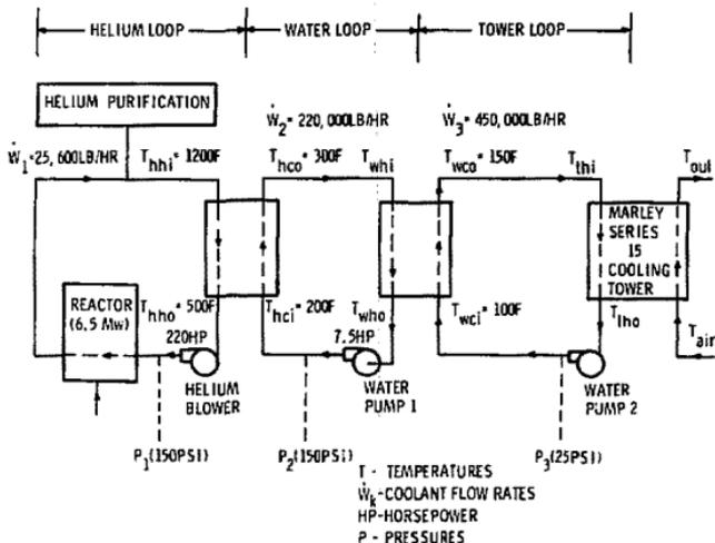
Figure 1. Cooling System Block Diagram
