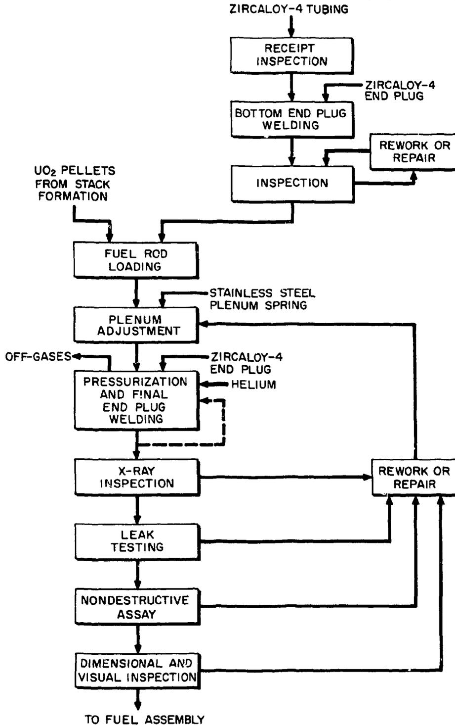
Fig. 3. Fuel Rod Fabrication Flowsheet.
