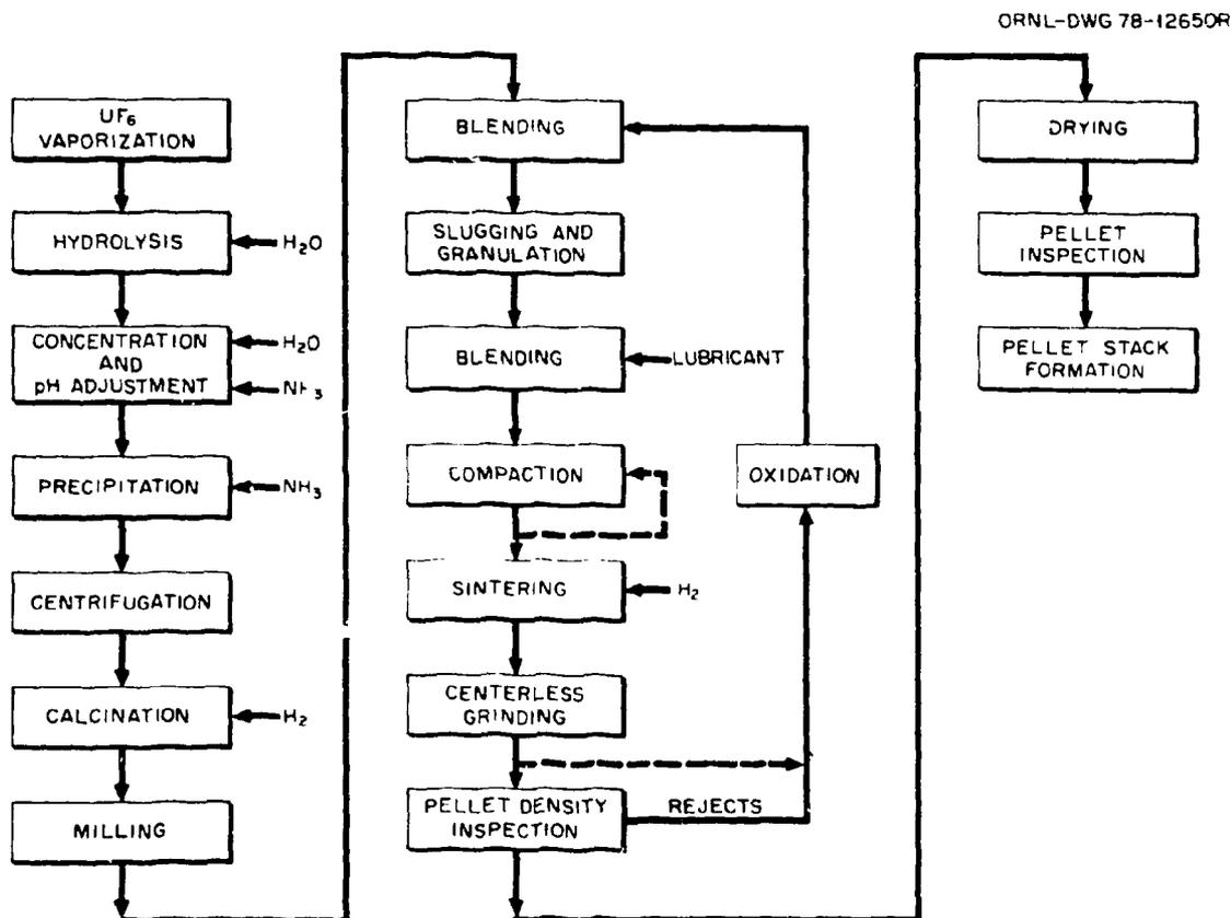
Fig. 2. Flowsheet of  $UO_2$  Pellet Fabrication.
