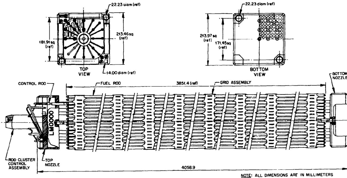
Fig. 1. Pressurized-Water Reactor Fuel Assembly with a 17 by 17 Rod Array.
