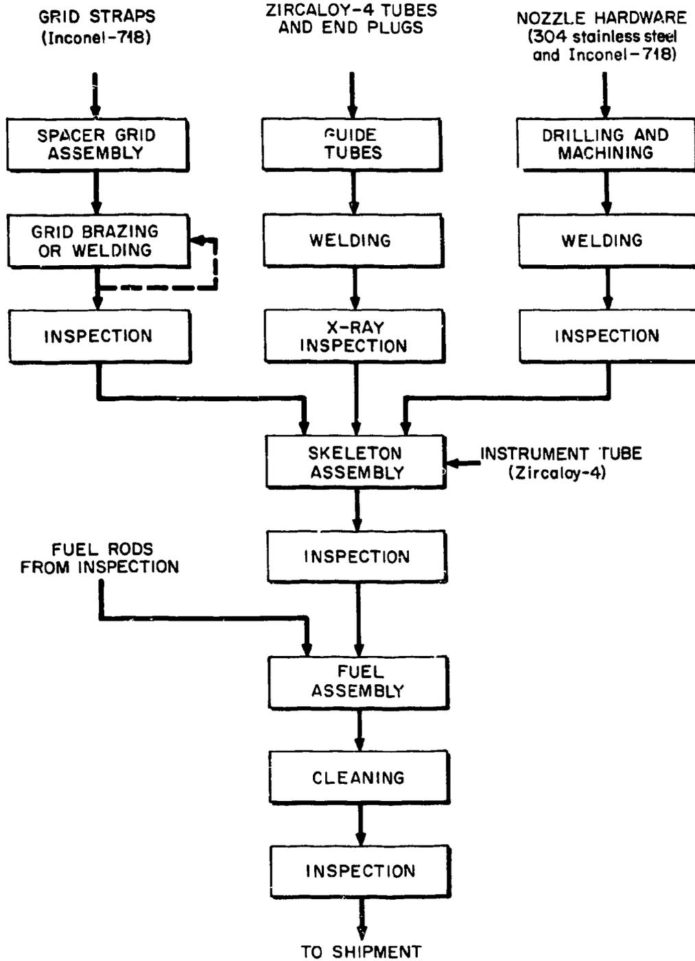
Fig. 4. Fuel Assembly Fabrication Flowsheet.
