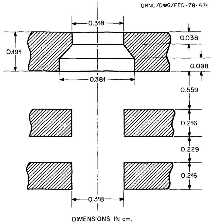
Fig. 2.3. Details of the shaped aperture.
