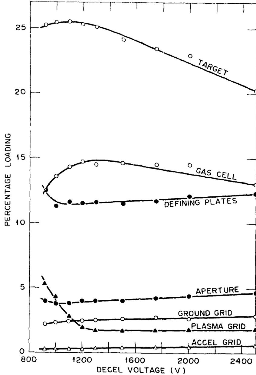
Fig. 4.4. Effect of varying the decel voltage on power deposition.
