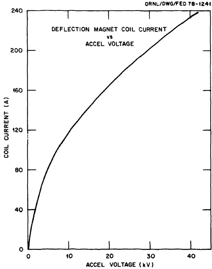
Fig. 2.4. The magnet current vs energy for hydrogen beam.
