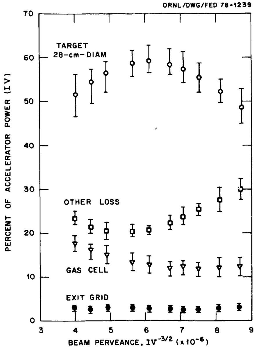
Fig. 4.5. Power deposition characteristics with shaped aperture grid.
