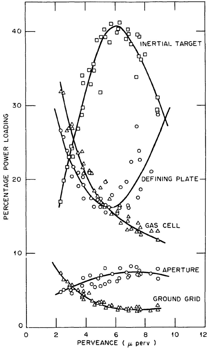
Fig. 4.1. Power deposition vs perveance without precel.
