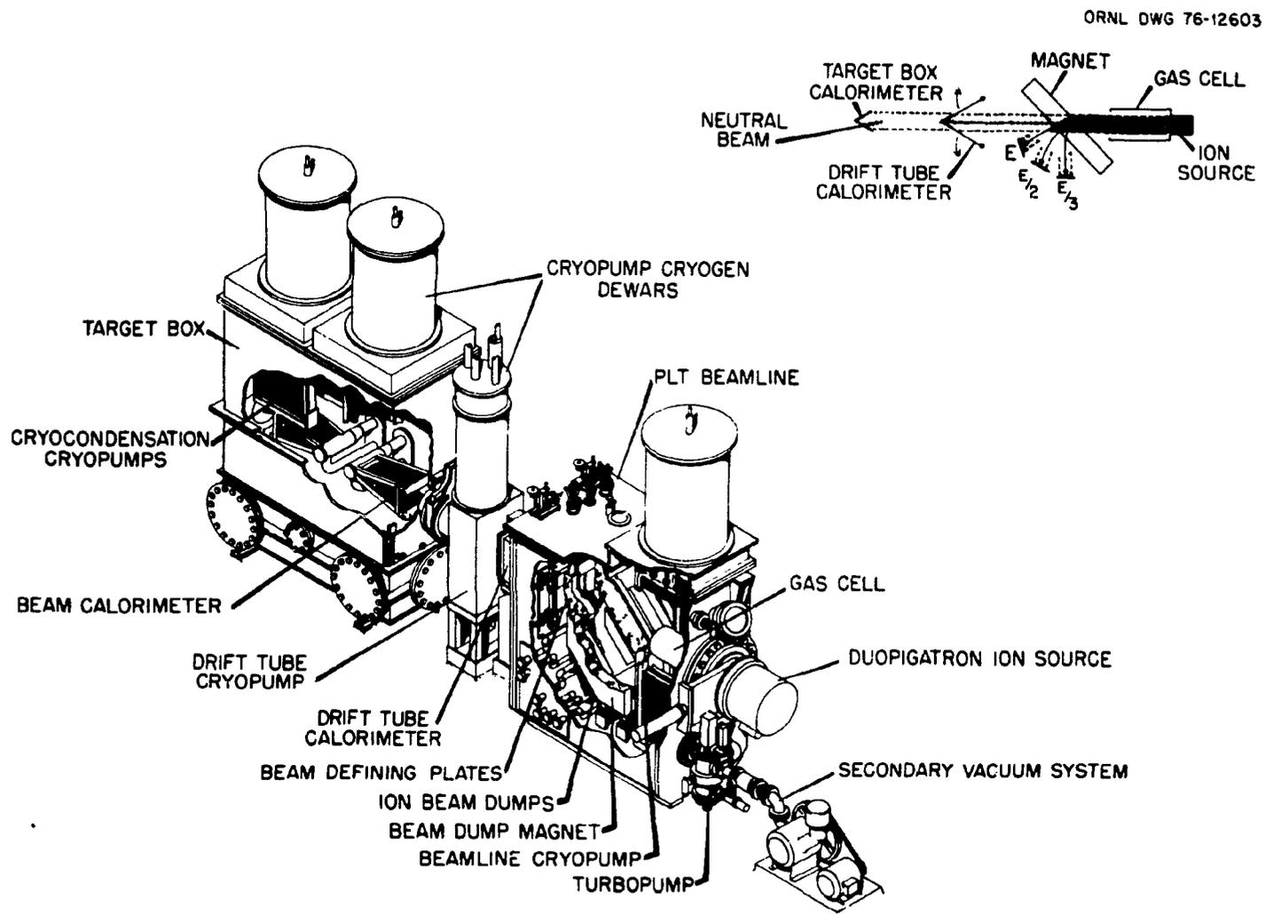
Fig. 2.1. ORNL/PLT beamline and target box.
