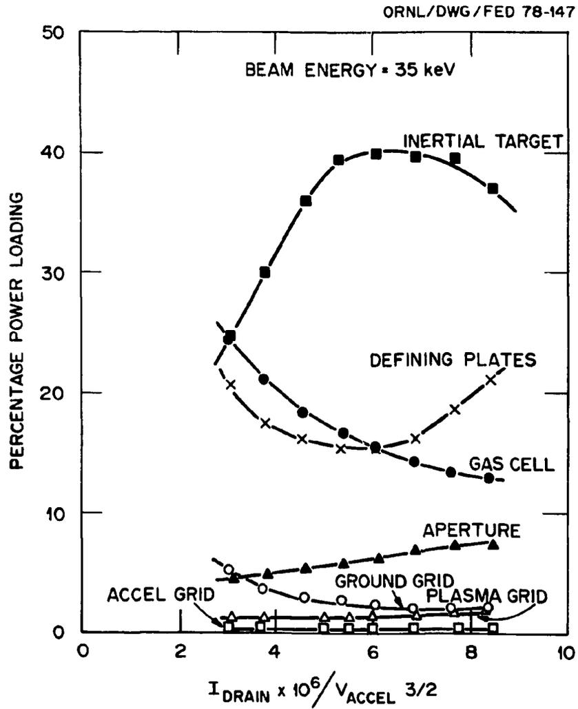
Fig. 4.3. Power deposition vs perveance at constant energy.
