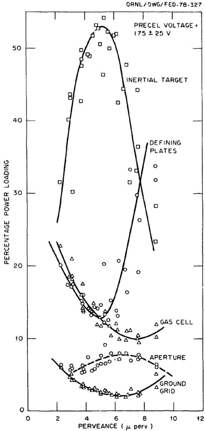
Fig. 4.2. Power deposition vs perveance with precel.
