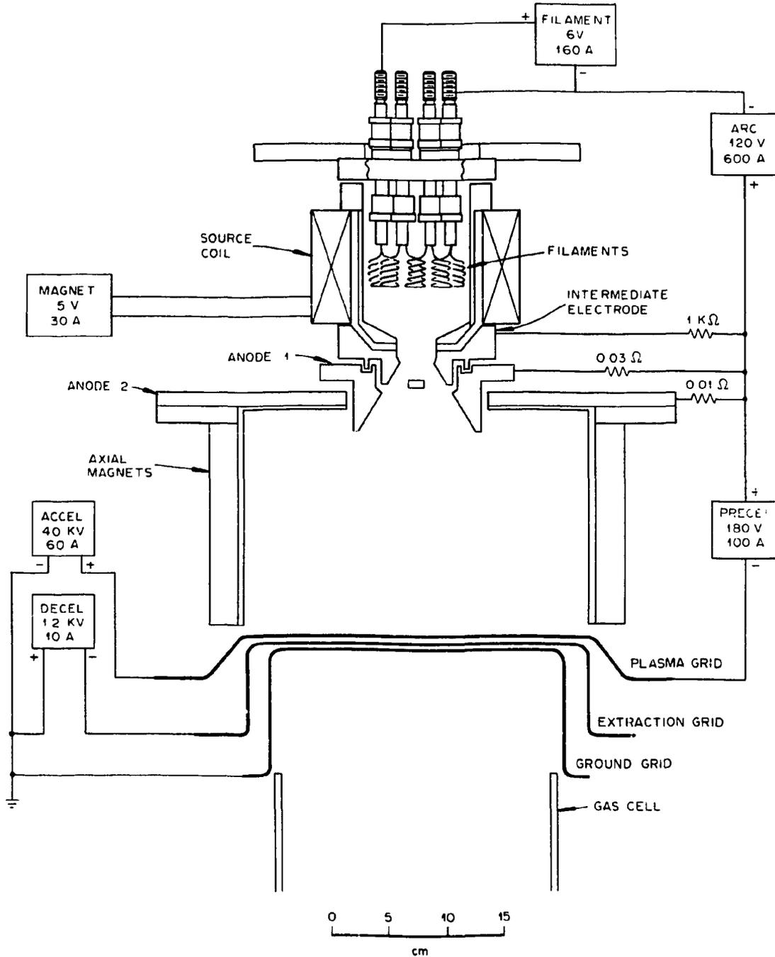
Fig. 2.2. Schematic representation of the ion source.
