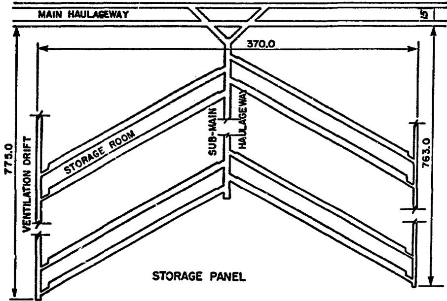
FIGURE 1: TYPICAL ROOM LAYOUT AND STORAGE PANELS (ALL DIMENSIONS IN METRES)
