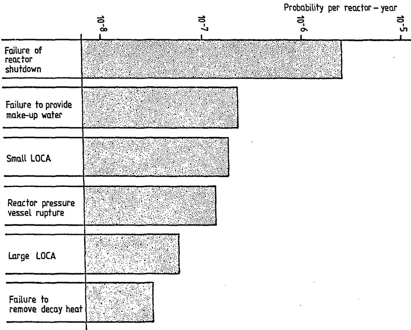
Figur 3 Probability of core melt in Forsmark 3
