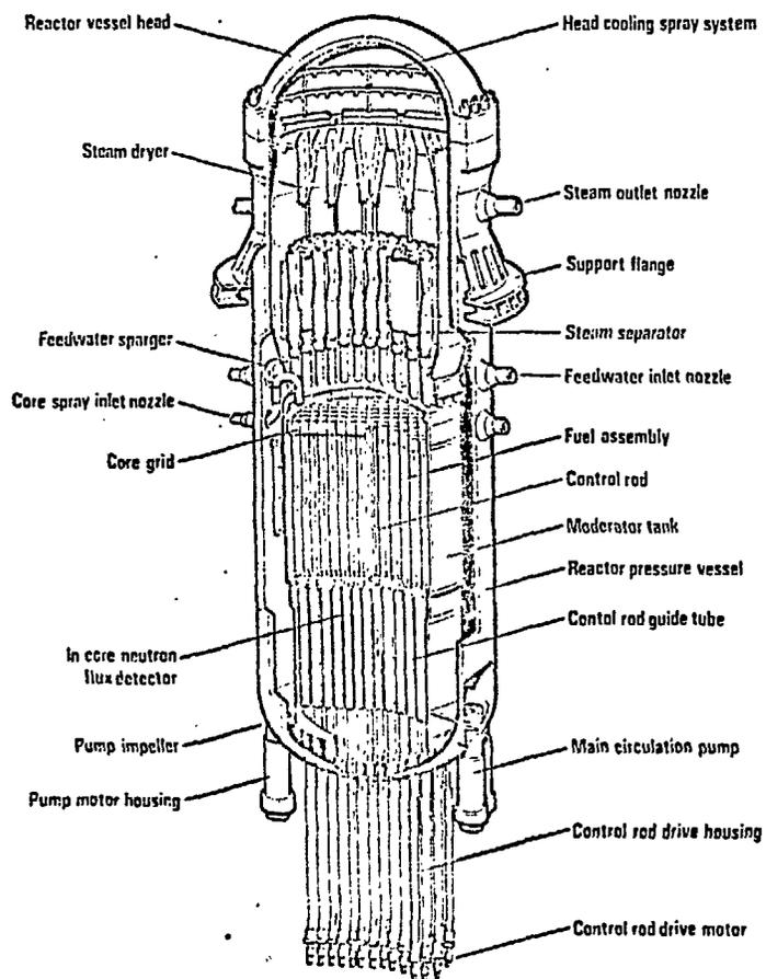
Figure 1. FORSMARK 3 - Reactor
