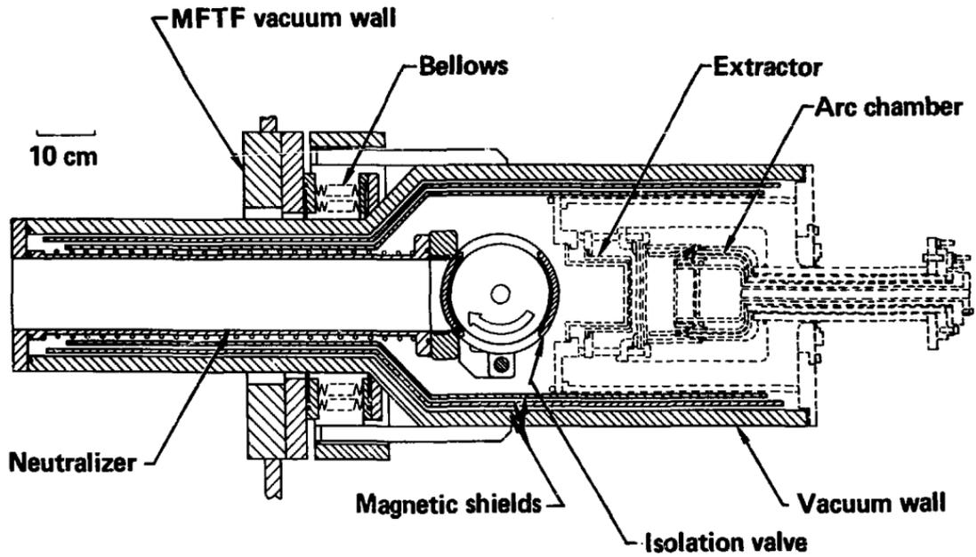
Figure 6. 80 keV MFTF source and injector module.
