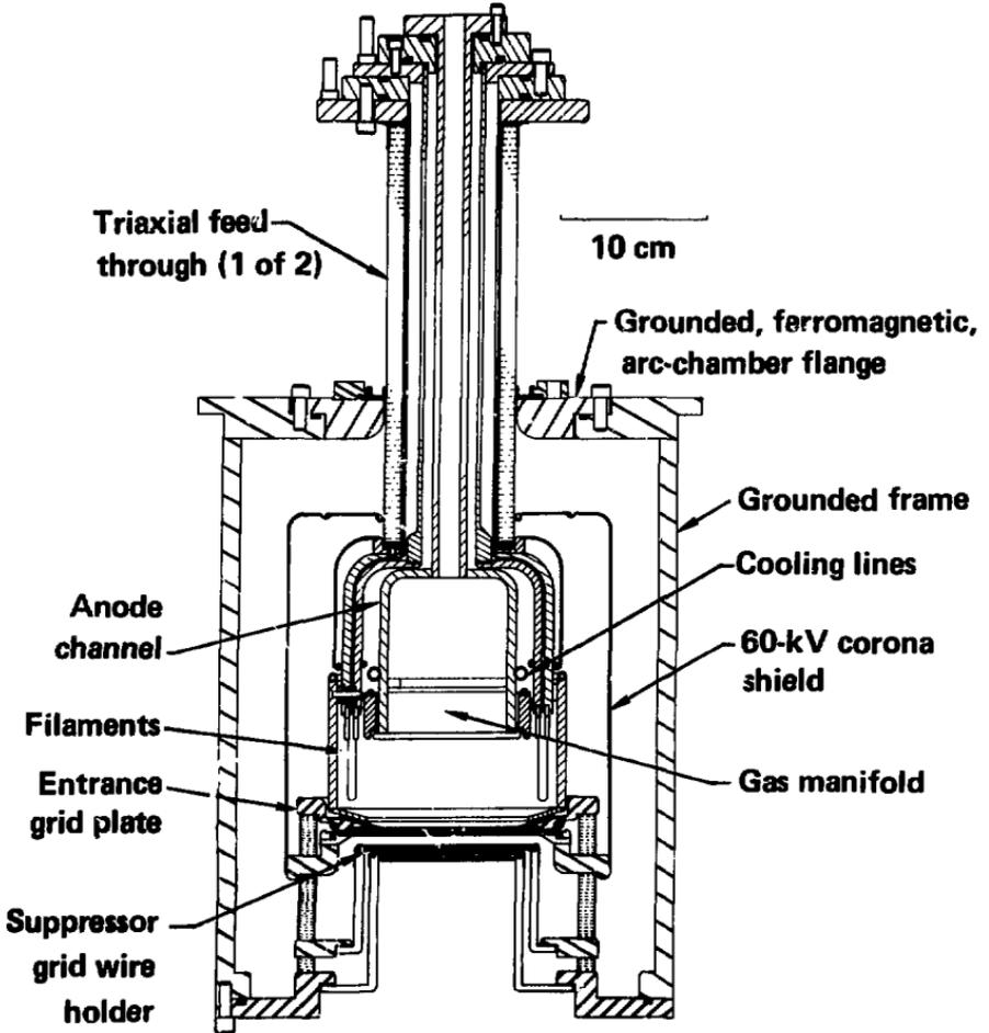
Figure 7. 80 keV neutral beam source.
