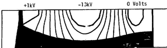
Figure 4. Accel-decel accelerator grid design used for producing 1-keV beams.
