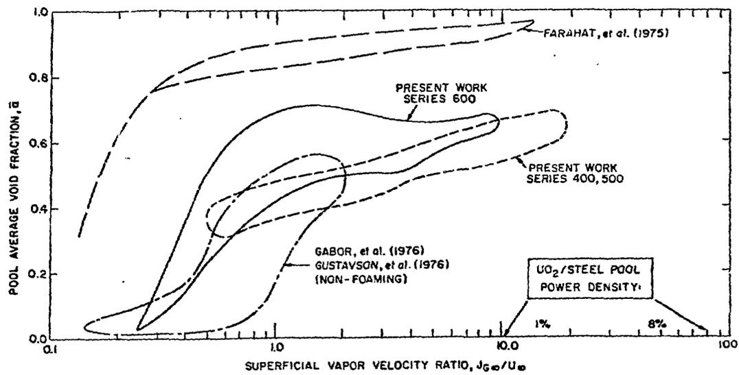
Figure 2.1 - Pool-Average Void Fraction Measurements
