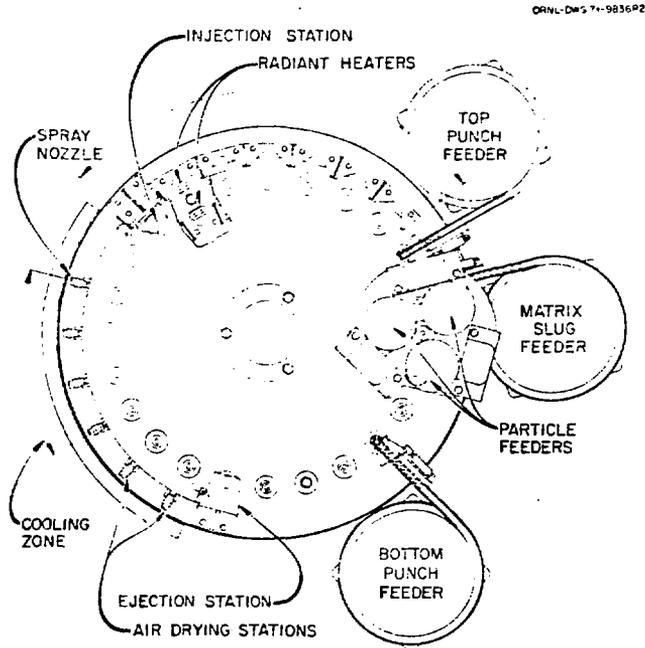
Fig. 2. Laboratory fuel rod molding machine schematic.
