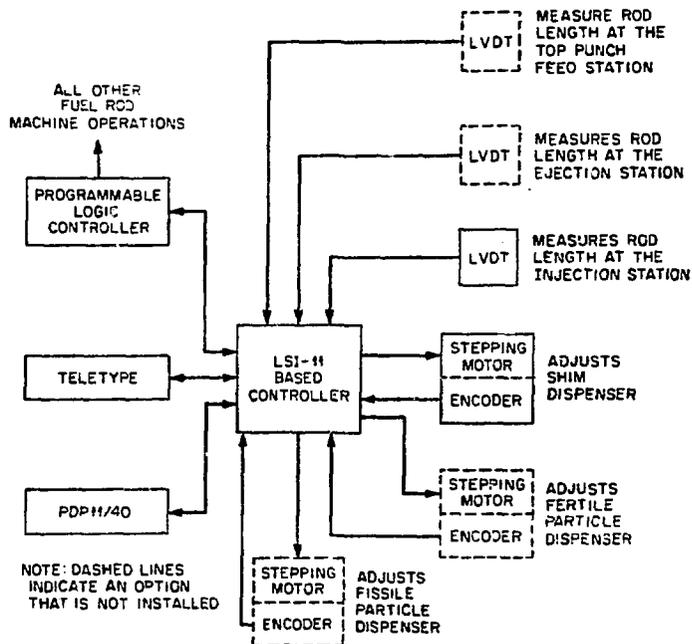
Fig. 6. Laboratory fuel rod molding machine control system block diagram.
