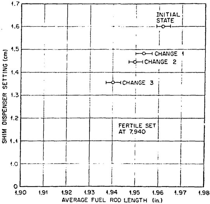
Fig. 4. Manually controlled shim dispenser setting vs fuel rod length.
