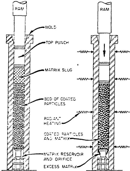
Fig. 3. Fuel rod molding components and technique for making bonded fuel rods.
