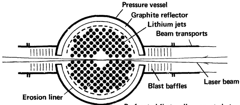
*Perforated first wall, supported at top and bottom and allowed to take transient stress in pure tension*
