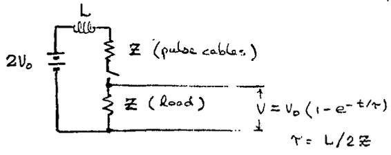
Figure 5 Equivalent Pulse Circuit
