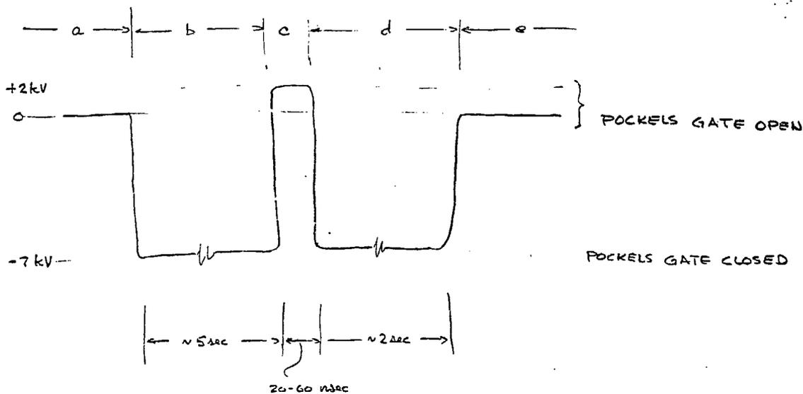
Figure 3 Voltage history of the pockels cell gate pulse:
