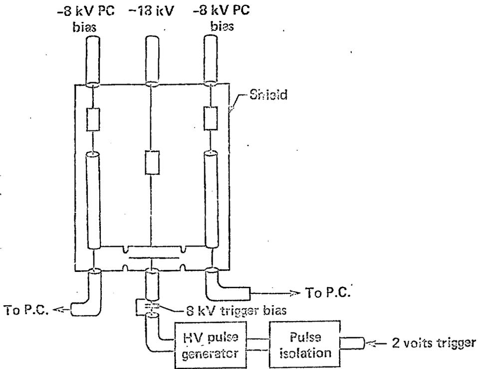
Figure 4. Arrangement of the Packets cell pulser using a mid-plane triggered spark gap switch.
