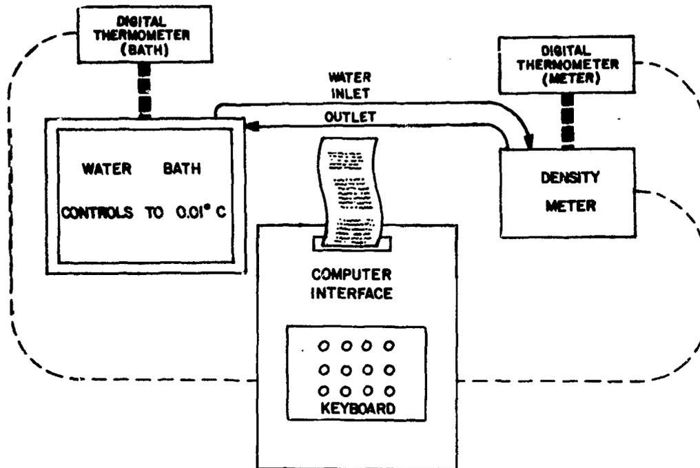
FIGURE 2 -- SCHEMATIC OF DENSITY MEASUREMENT SYSTEM
