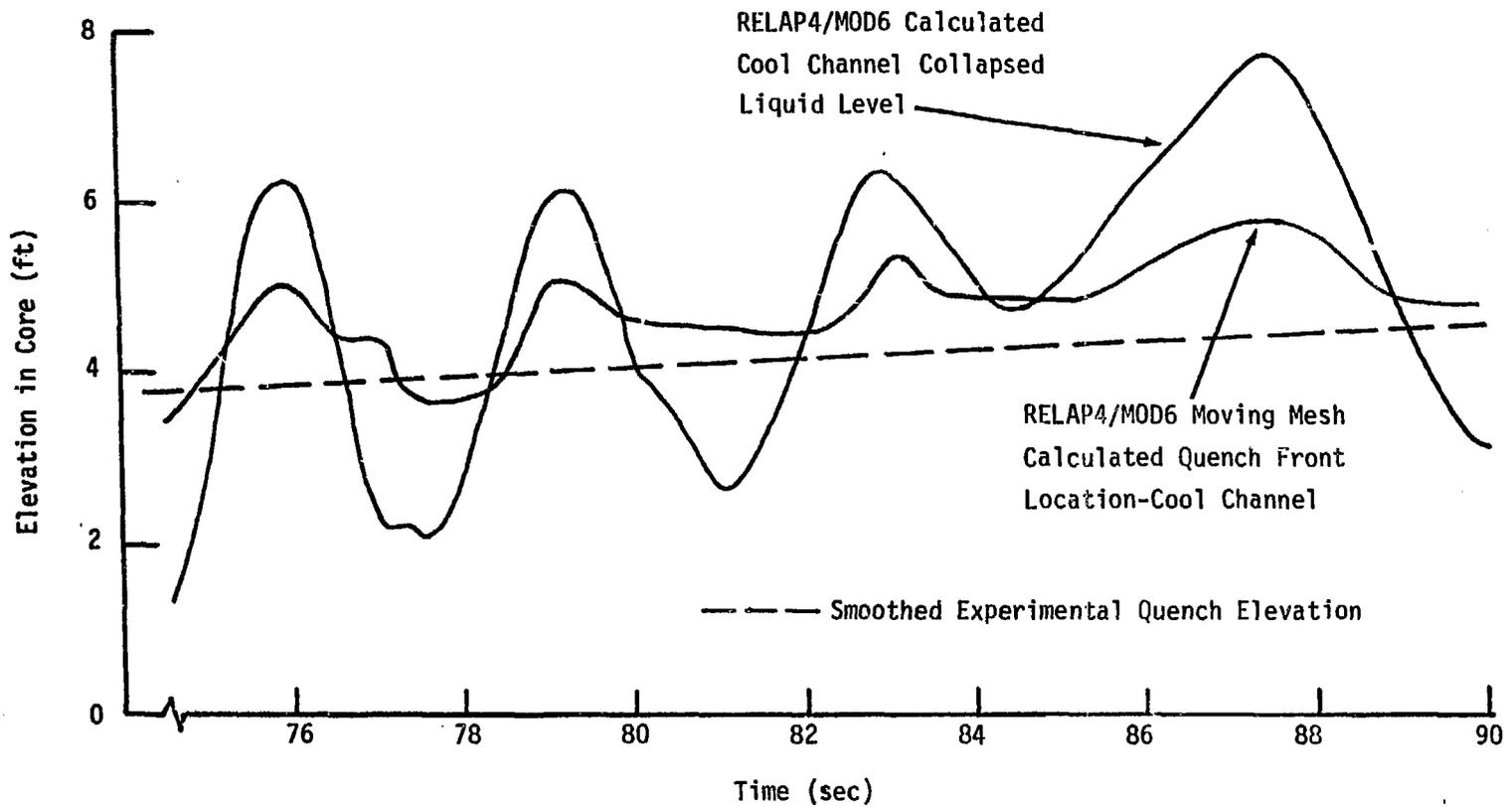
Fig. 2 Quench front propagation during reflood for PKL test K5A
