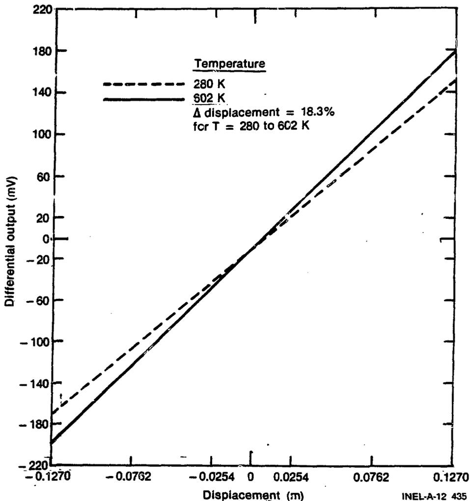
Fig. 3 Temperature sensitivity of the LVDT for temperatures of 280 and 602 K.
