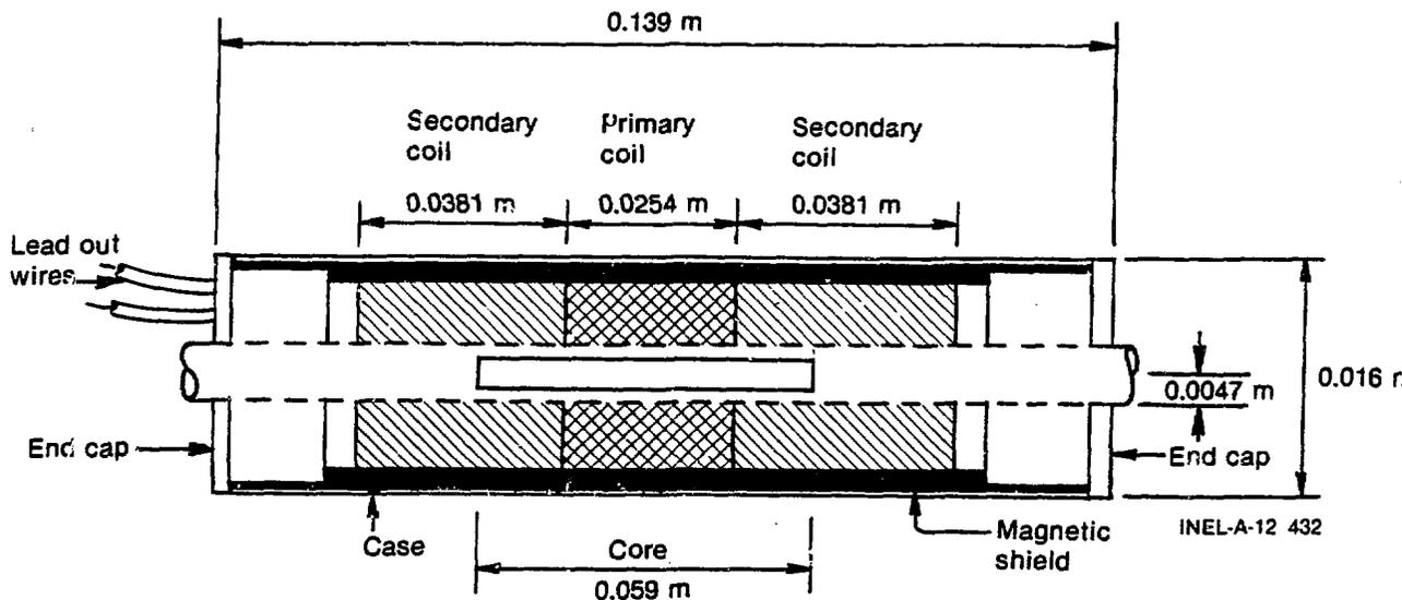
Fig. 2 LVDT used in the Power Burst Facility reactor.
