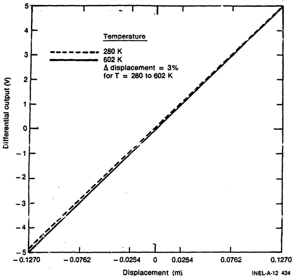
Fig. 5 Temperature sensitivity of the LVDT using compensating signal conditioning.
