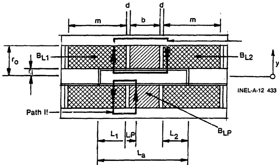
Fig. 1 Linear variable differential transformer model.
