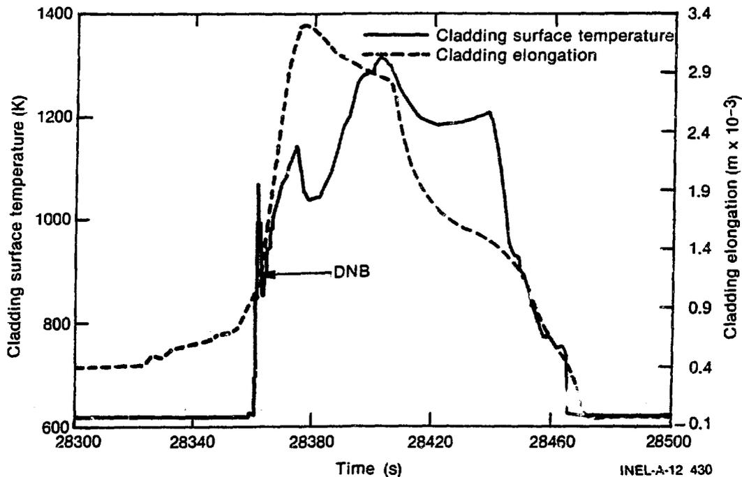
Fig. 8 Cladding surface temperature and cladding elongation as functions of time for Rod UTA-0008 during the final DNB cycle of Test PCM-2.
