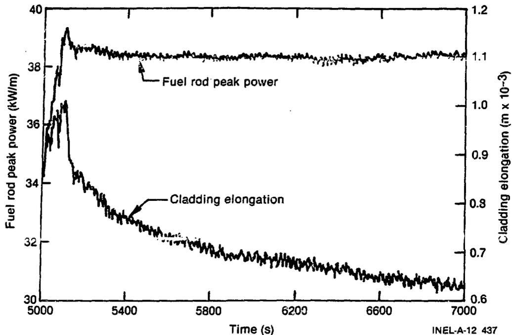
Fig. 7 Fuel rod peak power and cladding elongation as functions of time for Rod A-0014 during steady state operation in power calibration phase of Test PCM-2.
