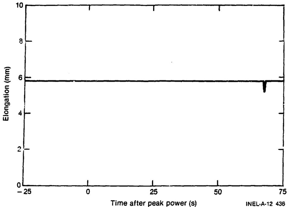
Fig. 6 Radiation sensitivity of the LVDT for RIA Scoping Test.
