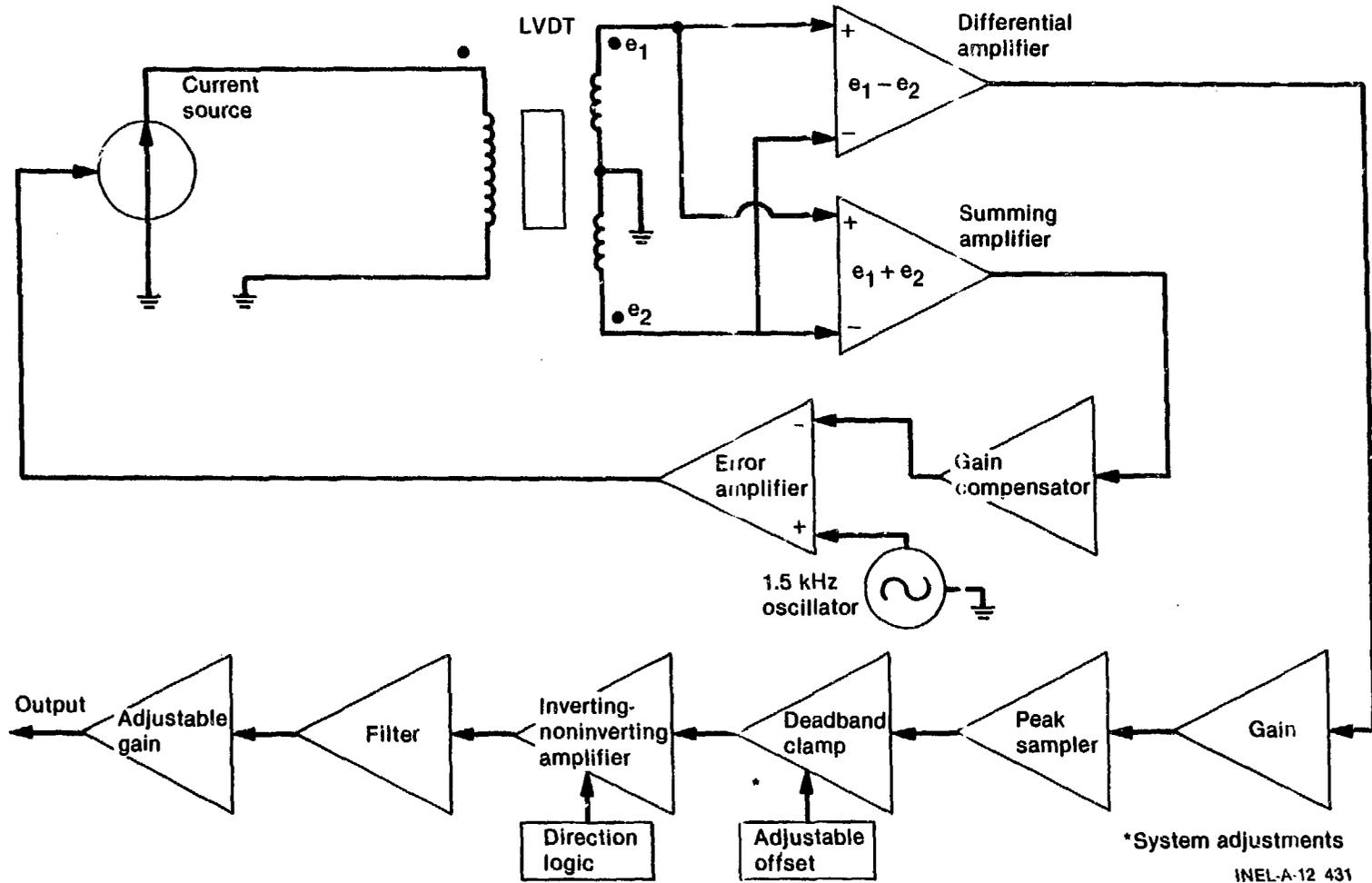
Fig. 4 LVDT temperature compensating electronics block diagram.
