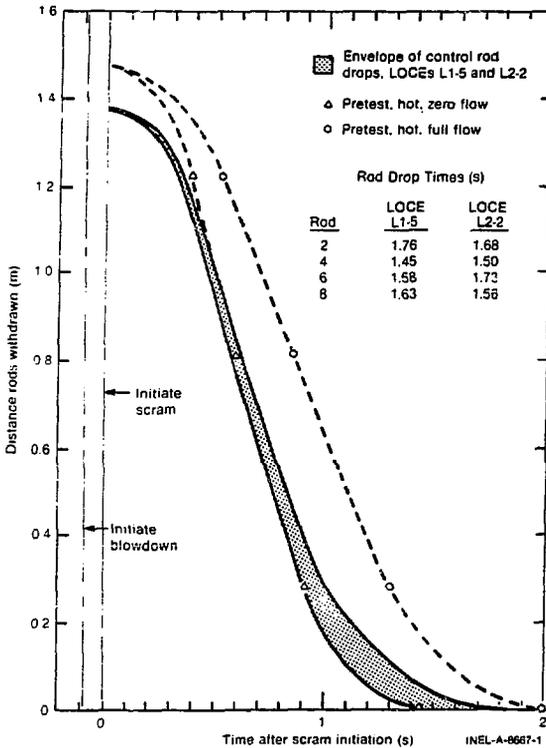
Fig. 4. - LOFT control rod drop times during LOCE scrams (rod position uncertainty of  $\pm 0.006$  m based on data from reed switch instrument supplier)
