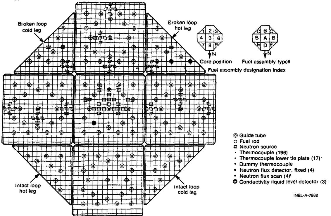
Fig. 2. - LOFT core configuration and instrumentation location
