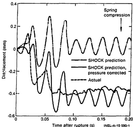
Fig. 3. - Center fuel module holddown spring displacement during LOCE L1-5 subcooled blowdown (uncertainty analysis for displacement data is contained in Reference 8)
