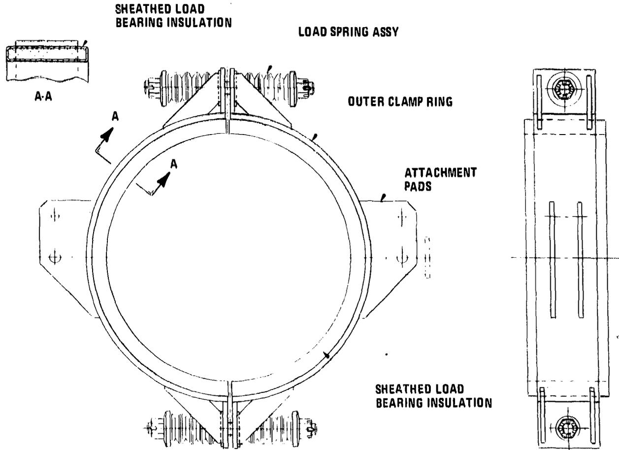
FIGURE 5: Horizontal Pipe Clamp Assembly
