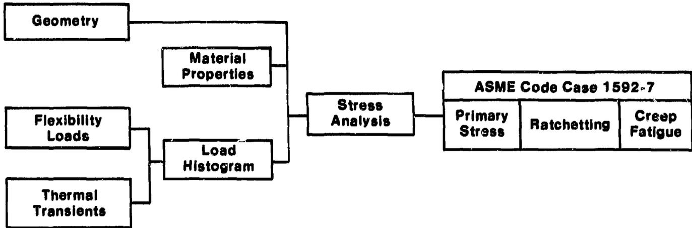
Figure 1. Piping Elastic Analysis Process
