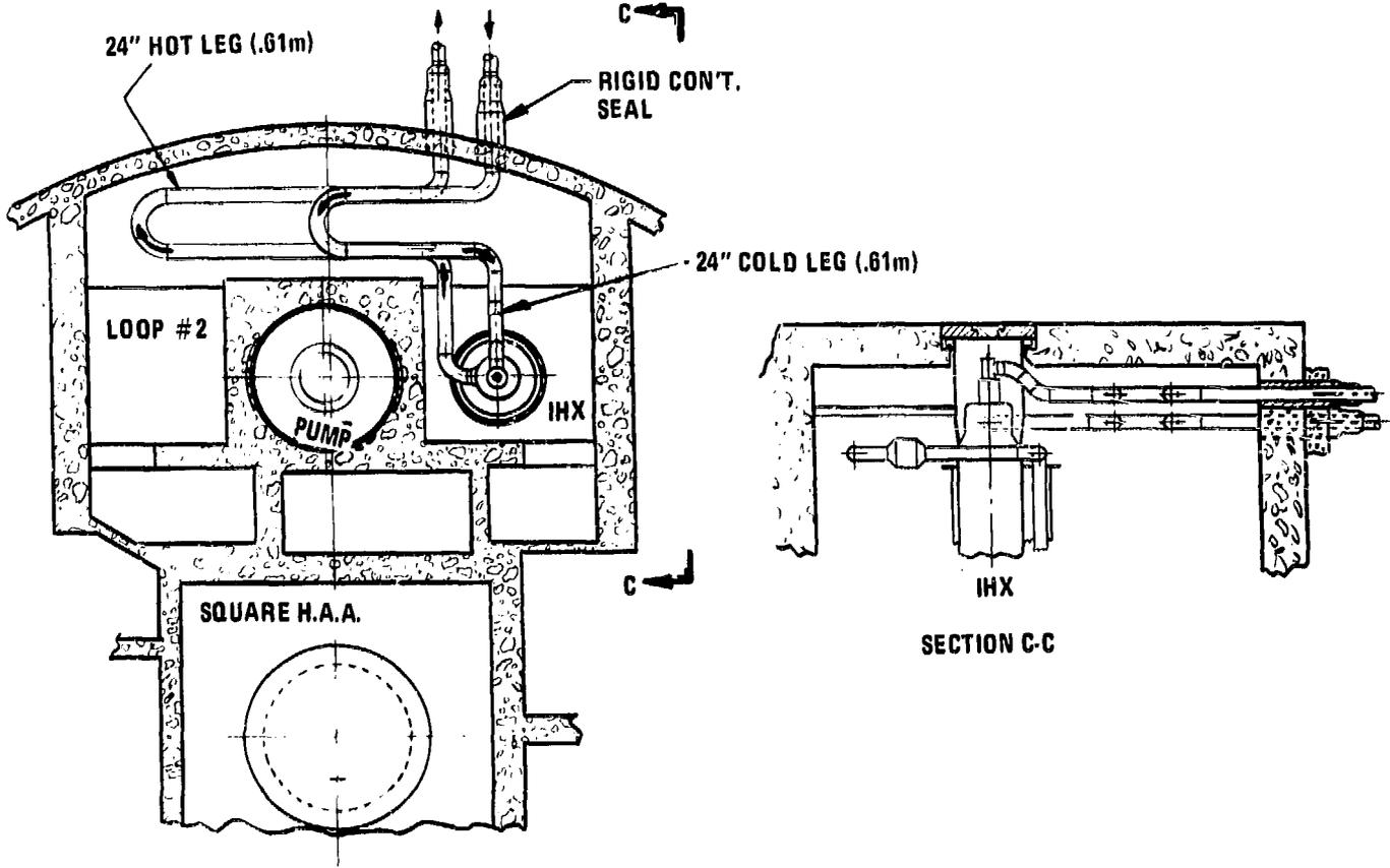
**IN CONTAINMENT INTERMEDIATE HEAT TRANSPORT SYSTEM PLAN ARRANGEMENT**
