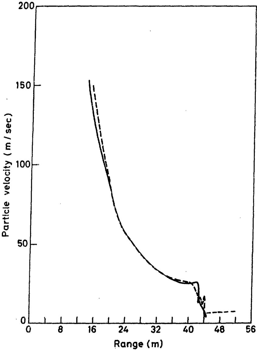
Fig. 7. Particle velocity profiles at the time when the shock reaches surface ground zero. —our calculation, ---Cherry's (1967) calculation.
