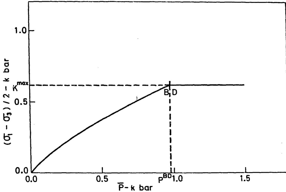
Fig. 5. A typical shear strength curve
