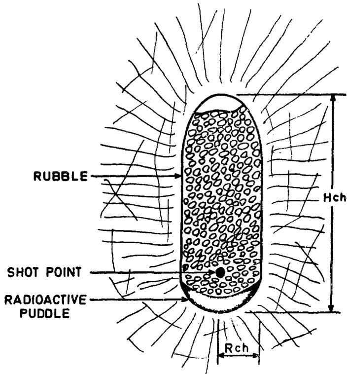
Fig. 1. Cross section of a chimney produced in hard rock for a deeply buried nuclear explosion.
