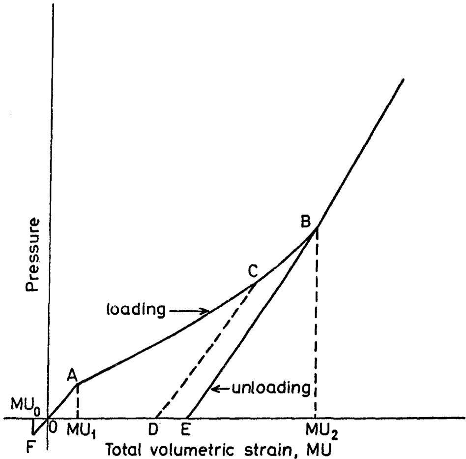
Fig. 4. Typical loading and unloading curve in  $P$ - $MU$  plane.  $MU_0$  is the bulking strain.  $MU_1$  is the strain upto which material is to be treated elastically and at  $MU_2$  the air filled porosity is completely removed.
