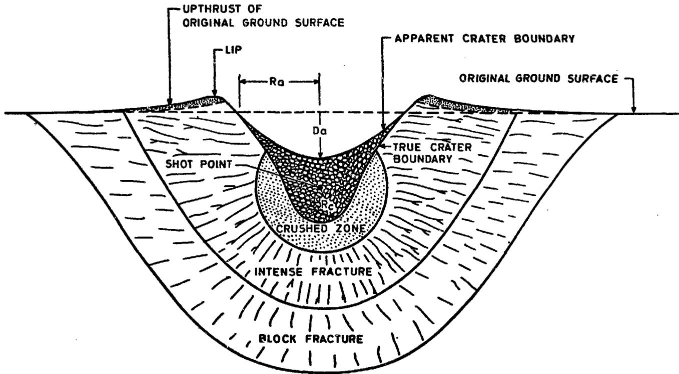
Fig. 2. Cross section of a crater produced by a nuclear explosion.
