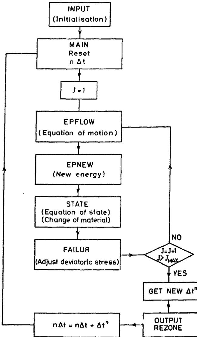
Fig. 3. Schematic flow diagram for the "OCENER" code
