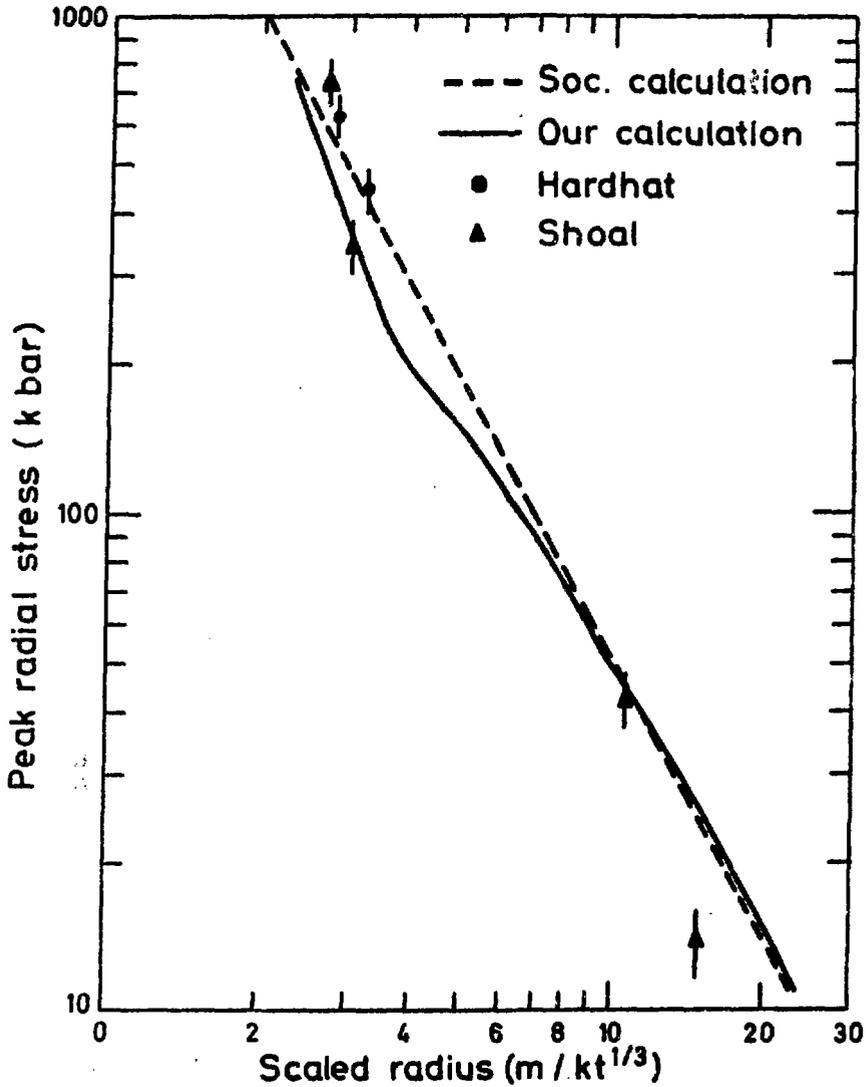
Fig. 6 Peak radial stress profile in granite
