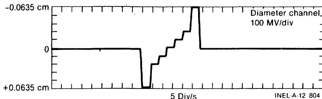
FIGURE 6--Diameter calibration data - LVDT system.
