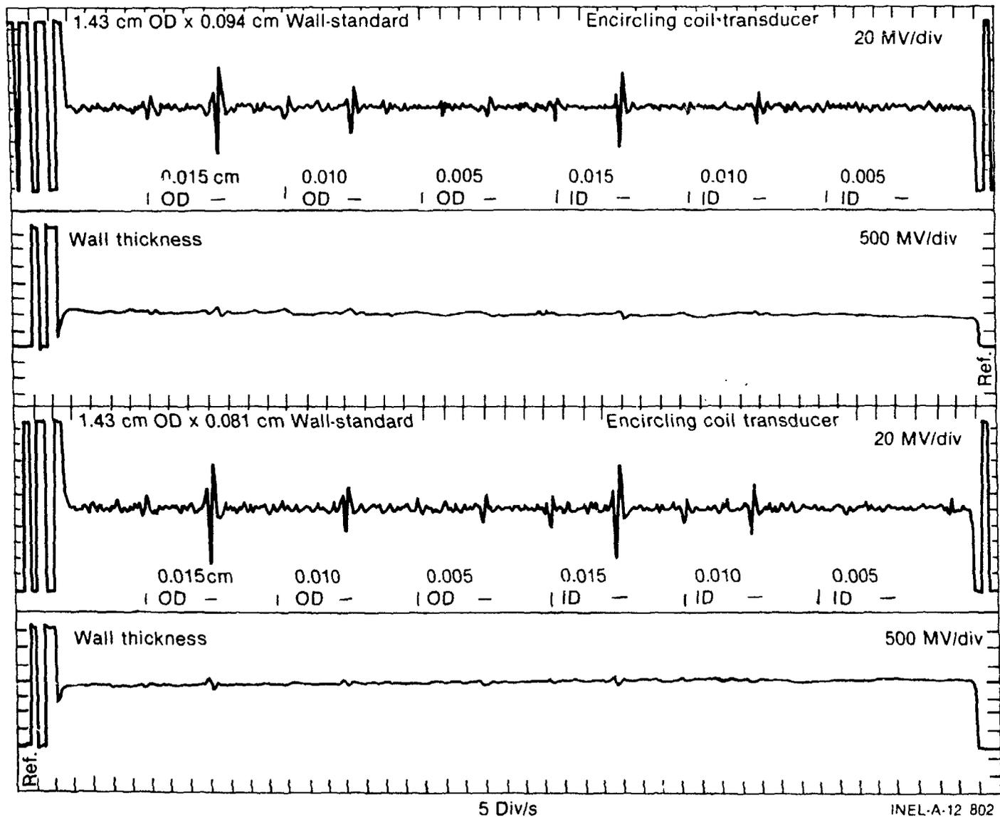
FIGURE 2--Response of encircling coil transducer to the defect standard.
