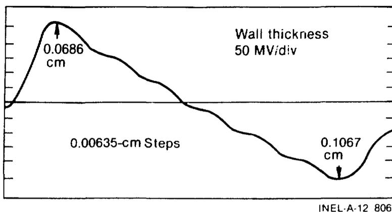
FIGURE 5--Response of point probe wall thickness transducer to the wall thickness standard.
