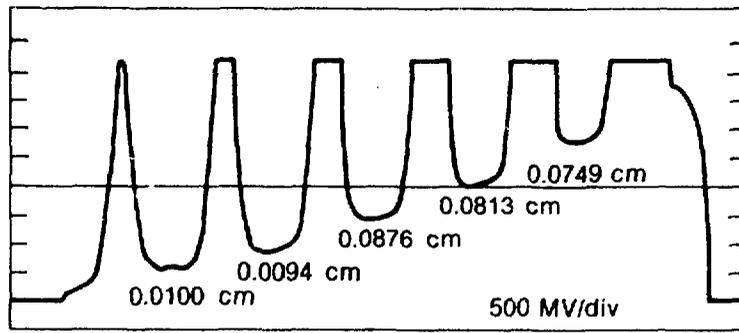
FIGURE 3--Response of encircling coil transducer to the wall thickness standard.
