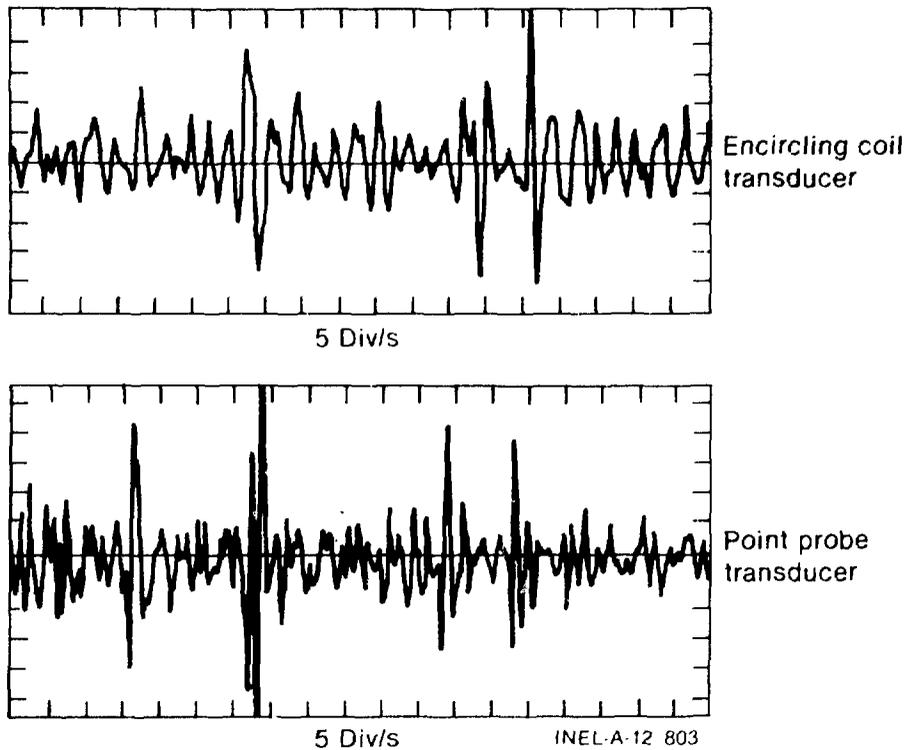
FIGURE 7--Actual fuel rod scan showing possible defects (fuel Rod ID-DA2999).
