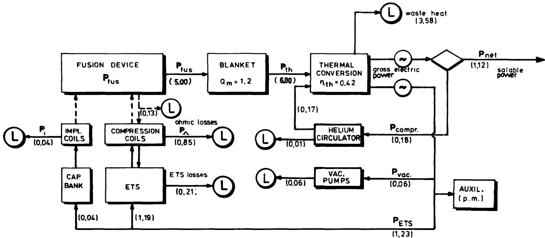
Fig. 3. Energy-flow diagram of the BSPR, data are given for the reference case in GW.
