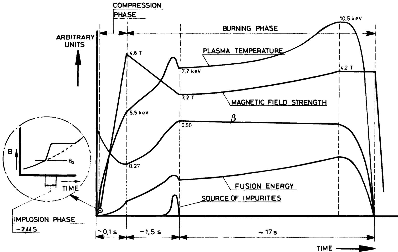
Fig. 2. Time dependence of the magnetic field strength, the temperature, the value of  $\beta$ , the produced fusion energy, and the number of injected impurity atoms.
