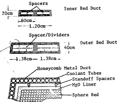
Fig. 8. High temperature reactor duct arrangement.
