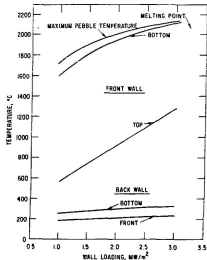
Fig. 4. Temperature profiles within an unimproved falling bed duct.
