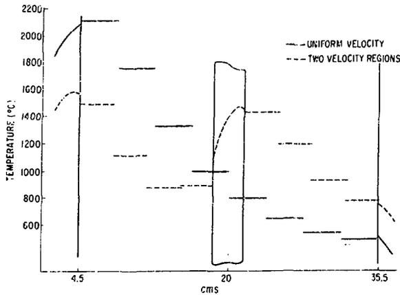
Fig. 5. The effect of velocity partitioning on the temperature profiles within a falling bed duct.
