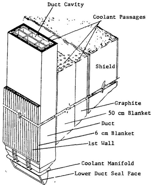
Fig. 7. Outer blanket duct arrangement.
