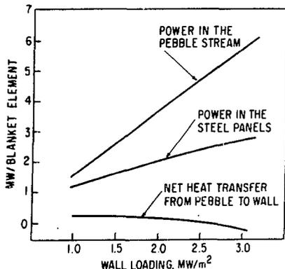
Fig. 3. The partitioning of power in an unimproved falling bed duct.
