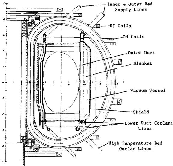
Fig. 2. A cross section of the high temperature tokamak reactor.
