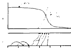
Fig. 7. The structure of the front in a MITL. The voltage and loss current density are shown in A and the electron map is shown in B. The pulse risetime is \sim 0.3 ns.
