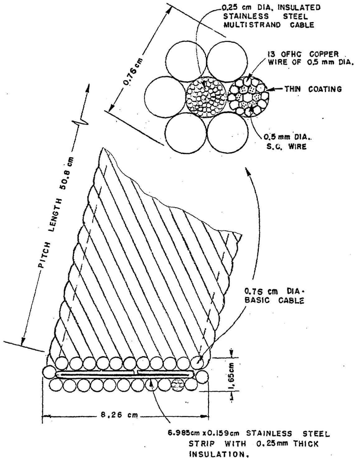
Fig. 8. 50-kA ac superconducting cable.
