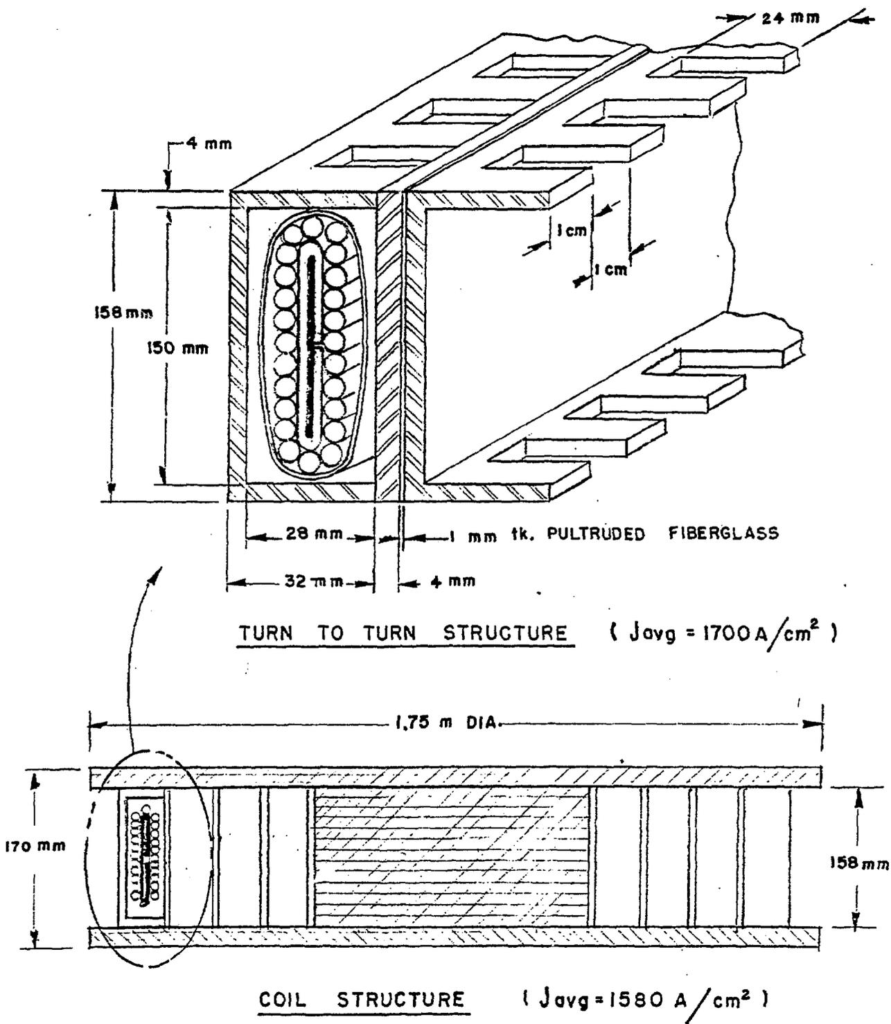
Fig. 10. Pulsed-coil structure.
