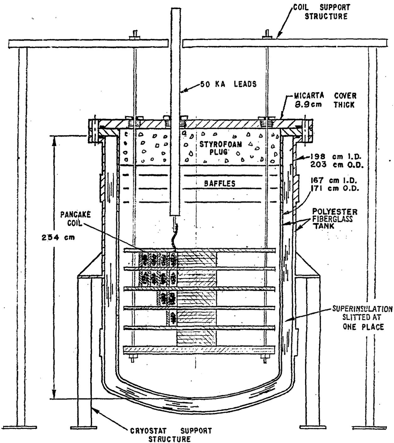
Fig. 11. Plastic dewar for high-current cable pancake coils.
