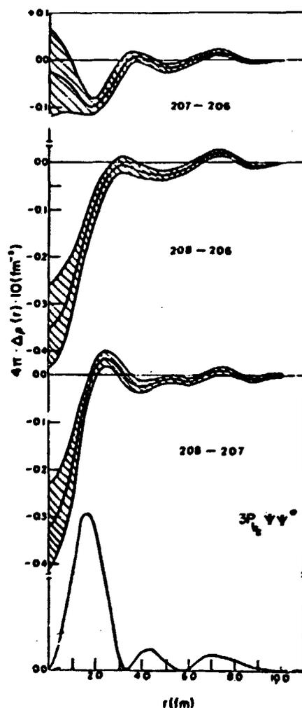
Fig. 12 -  $^{208}-^{207}\text{Pb}$ ,  $^{208}-^{206}\text{Pb}$ ,  $^{207}-^{208}\text{Pb}$  charge differences together with a  $3p_{1/2}$  neutron wave function predicted by a self consistent theory.
