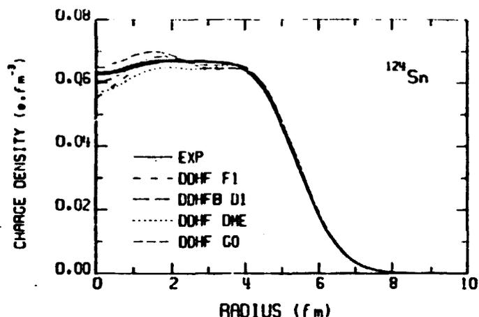
Fig. 11 -  $^{124}\text{Sn}$  charge density together with mean field predictions (F1 = Beiner-Lombard, D1 = Gogny, DME = Negele, GO = Campi-Sprung).
