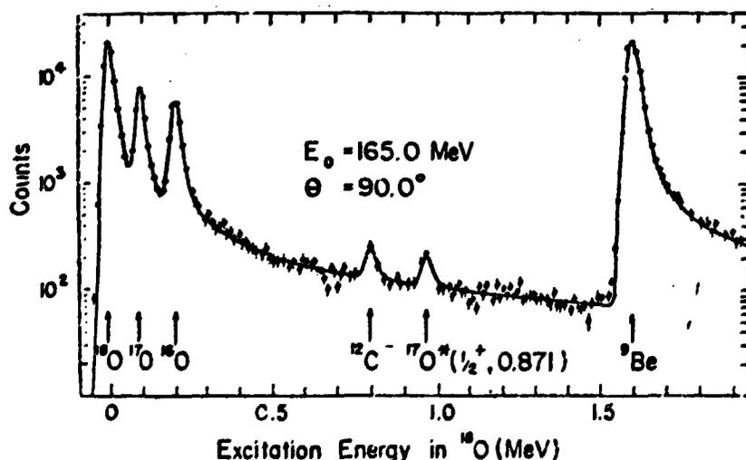
Fig. 4 - Typical spectrum for elastic scattering a from oxygen isotopes mixed in a BeO target.
