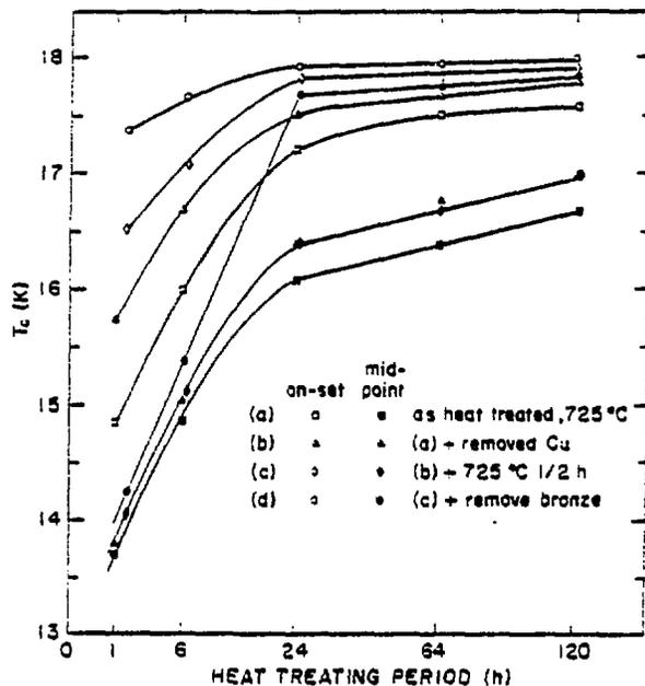
Figure 4. The variation in  $T_c$  after removal of the copper and the bronze matrices is shown as a function of heat treatment periods for the wire FM 102.
