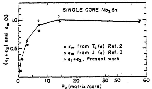
Figure 7. The axial strains, ( $\epsilon_1+\epsilon_2$ ), in the monofilamentary wires ( $R_v=15$ ), calculated from Eq. (2), are compared with those strains determined from the in-situ application of tensile strains for  $T_c$  and  $J_c$  measurements.
