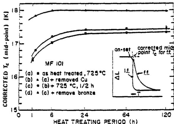
Figure 3. The variation in  $T_c$  after removal of the copper and the bronze matrices is shown as a function of heat treatment periods for wire FM 101. The determination of the midpoint  $T_c$  is defined in the insert.
