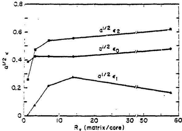
Figure 6. The calculated parameters,  $a/2\epsilon_0$ ,  $a/2\epsilon_1$ , and  $a/2\epsilon_2$ , which are proportional to the strains in  $Nb_3Sn$  from disorder, the plastic strain in Nb, and the bronze matrix, are shown as a function of the volume ratio  $R_v$  for the monofilamentary wires.
