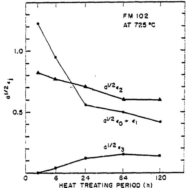
Figure 8. The strain parameters,  $a/2\epsilon_1/2$ ,  $a/2\epsilon_2$ , and  $a/2\epsilon_3$ , for FM 101 are shown as a function of heat treatment time.
