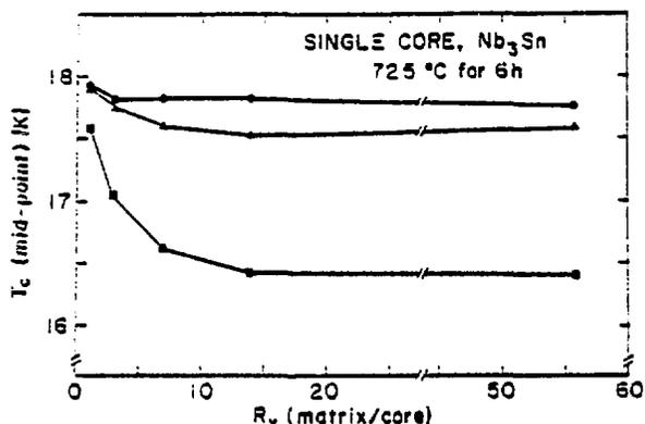
Figure 5. The effect of the variation in the matrix to the core ratio  $R_v$  on  $T_c$  after removal of the matrix and following annealing (0.5 h at 725°C) is illustrated for the monofilamentary wires heated for 16 h at 725°C.
