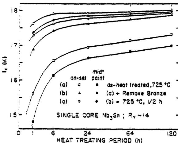
Figure 2. The variation in  $T_c$  after removal of the bronze matrix and following the annealing treatment (0.5 h at 725°C) as a function of heat treatment periods is shown for the monofilamentary wire with a bronze to core ratio of 14.
