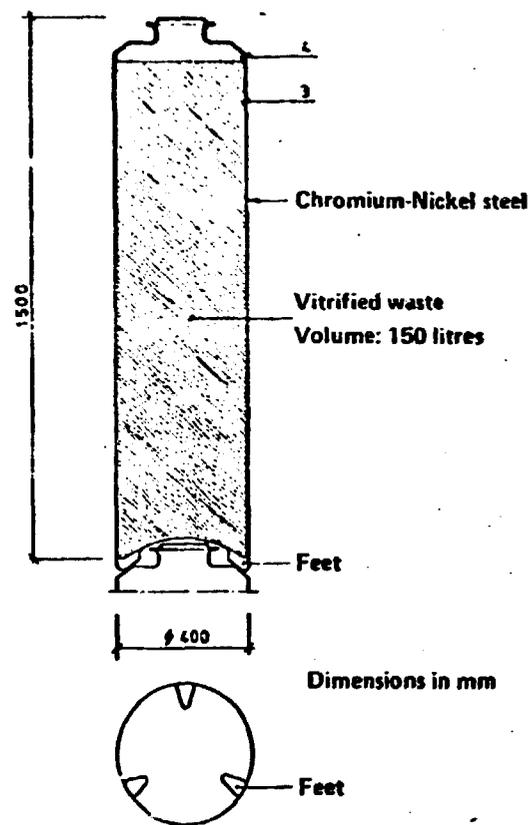
*Waste cylinder. The vitrified waste is cast in a container made of chromium-nickel steel. The container is sealed with a welded-on lid. The feet enable the waste cylinders to be stacked on top of each other.*
