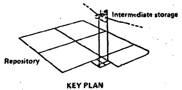
*Perspective drawing of plant for intermediate storage and encapsulation. It is located underground with a rock cover approximately 30 metres thick. The plant is located above the final repository.*
