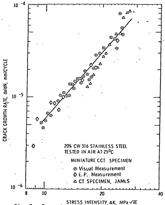
Fig. 7: Comparison of Room Temperature Fatigue Crack Growth Rates for CCT Specimen (e.p. and Visual Measurements) and CT Specimen (Visual), James.<sup>9</sup>
