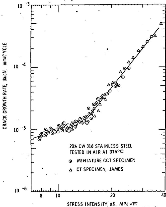
Fig. 8: Comparison of Elevated Temperature FCP for CCT Specimen (e.p. Method) and CT Specimen (Visual Method), James.<sup>9</sup>
