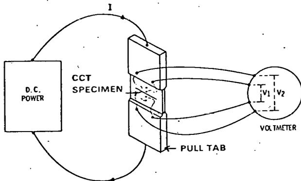
Fig. 3: Electrical Potential Measurement Details
