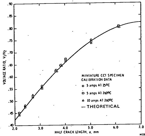
Fig. 4: Calibration Curve, Voltage Ratio Versus Half Crack Length
