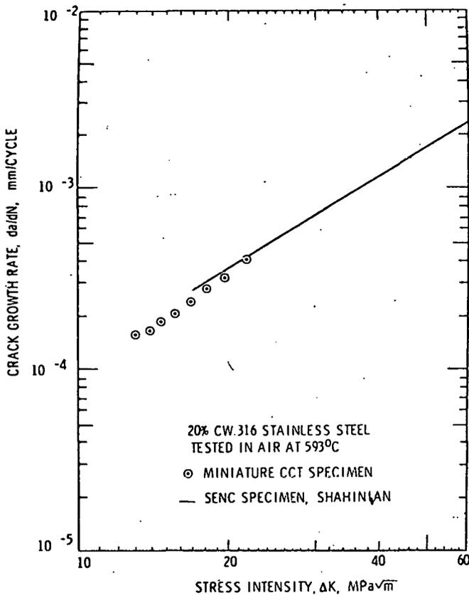
Fig. 9: Comparison of Elevated Temperature FCP for CCT Specimen (e.p. Method) and SENC Specimen (Visual Method), Shahinian.<sup>10</sup>
