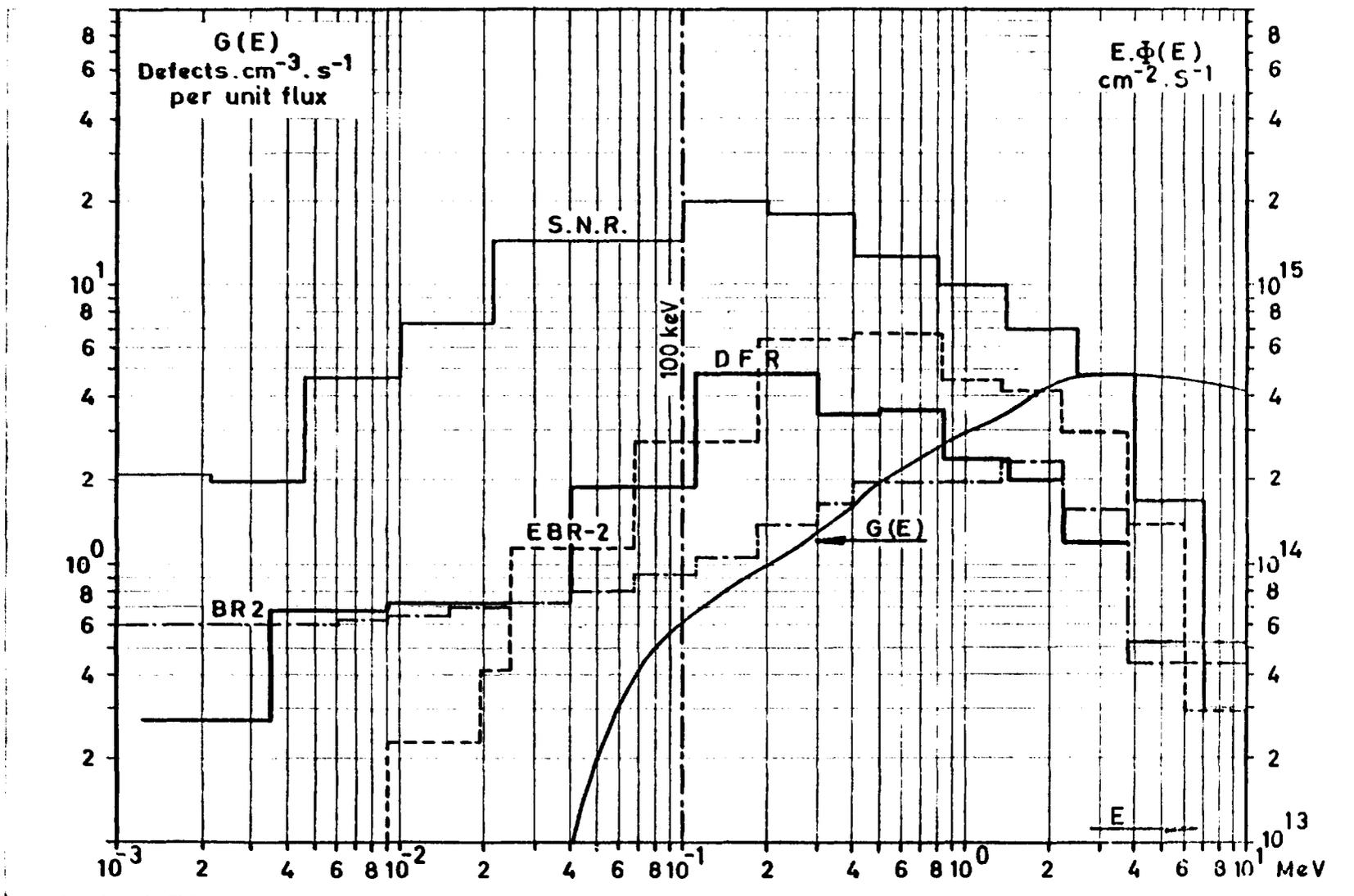
Fig. 10 Neutron spectra in various reactors and steel damage function.
