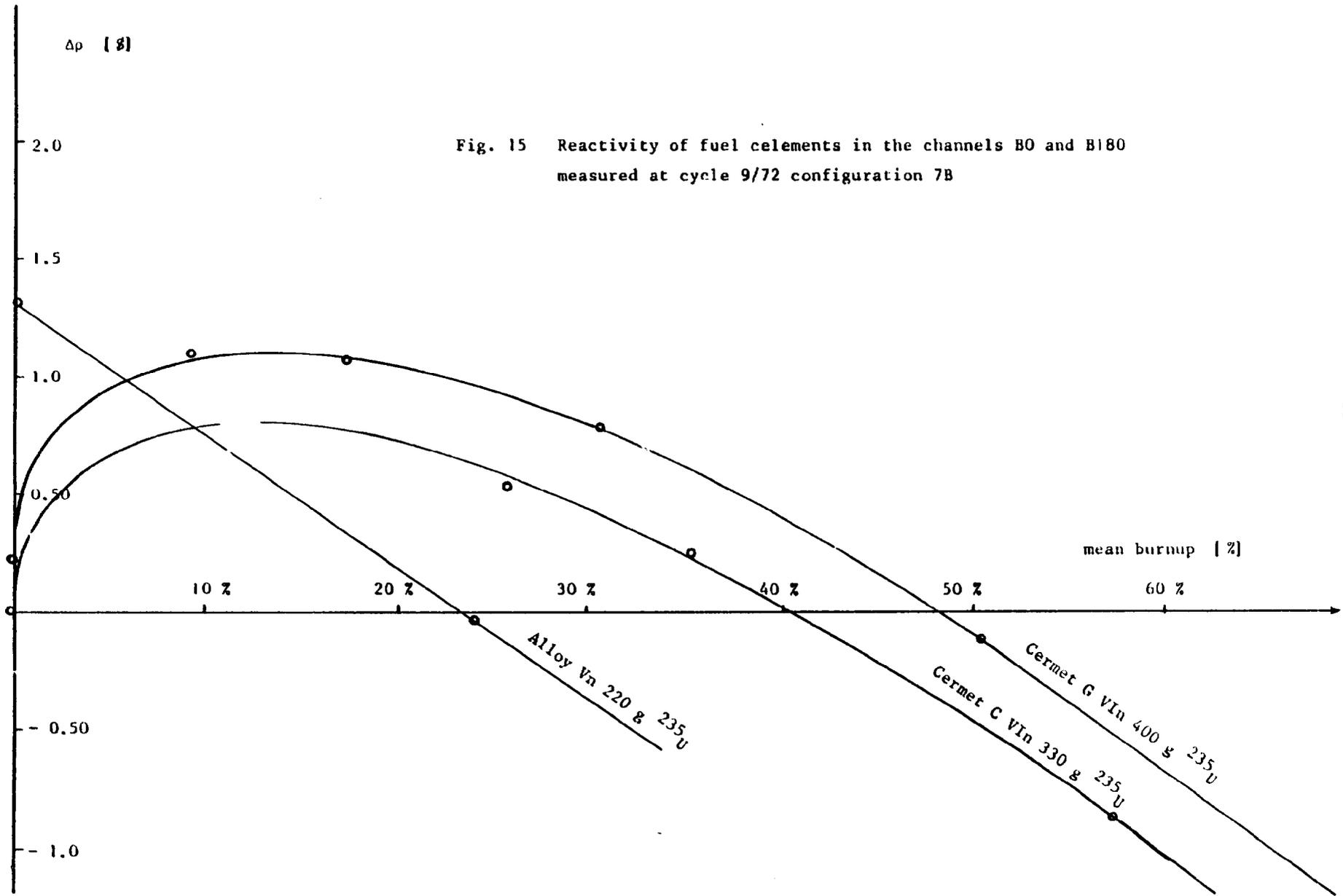
Fig. 15 Reactivity of fuel elements in the channels B0 and B180 measured at cycle 9/72 configuration 7B
