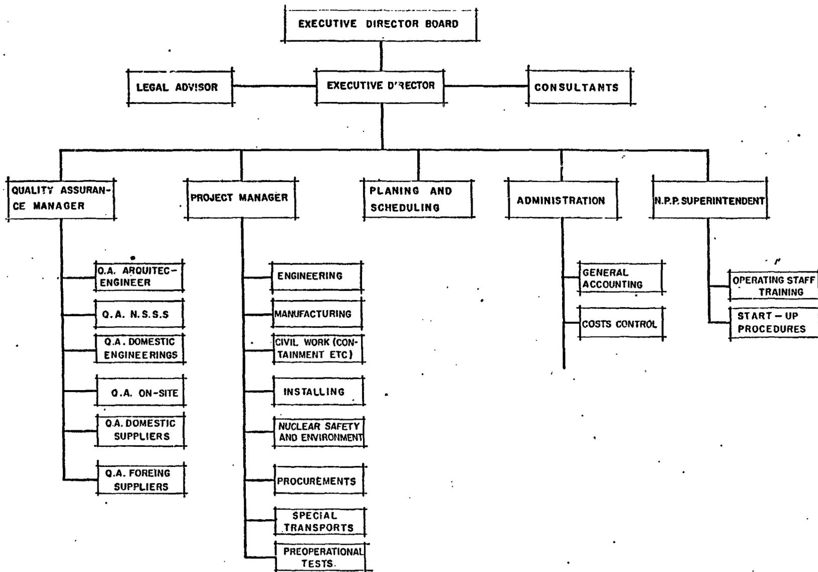
FIG. 1.—BASIC NUCLEAR POWER PROJECT PLANNING AND CONSTRUCTION ORGANIZATION CHART.
