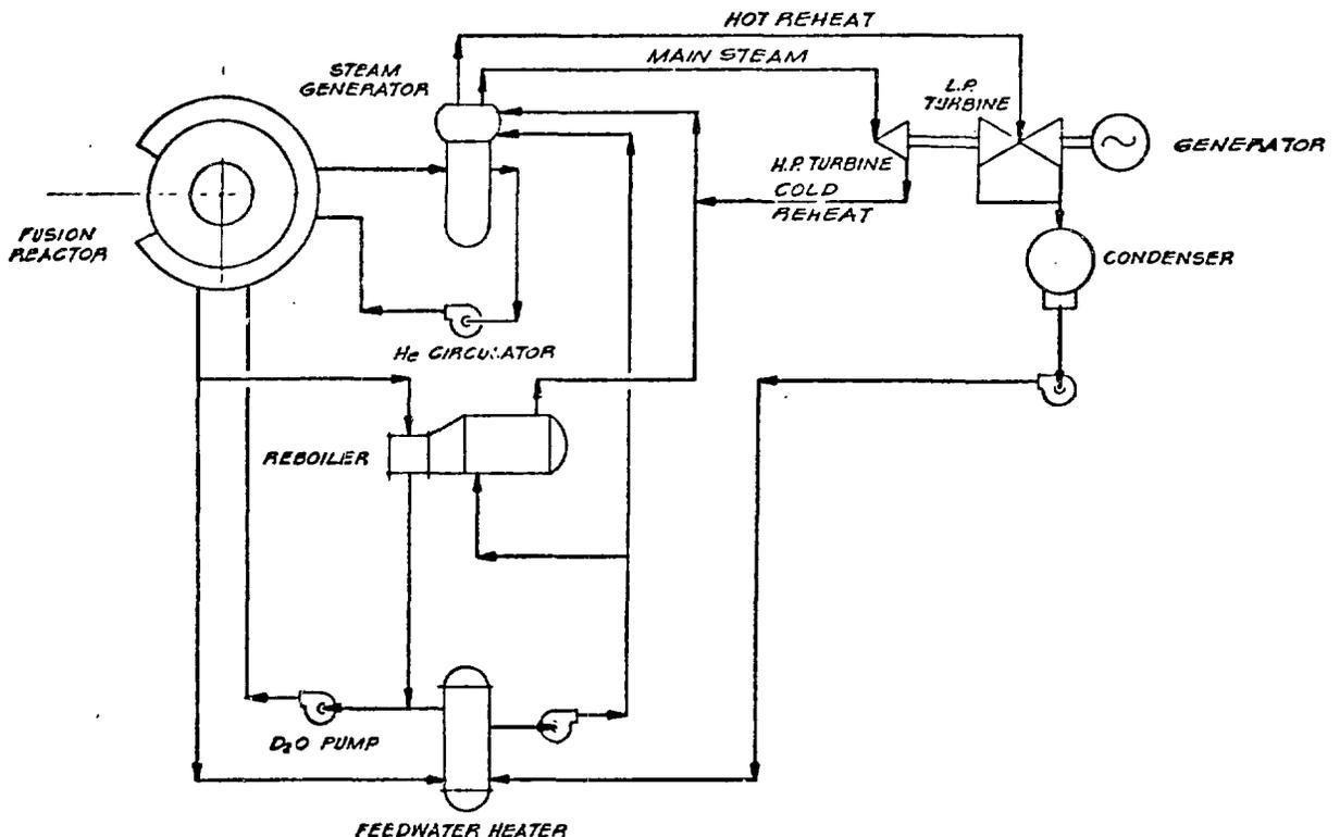
Figure 2. Power conversion system schematic.
