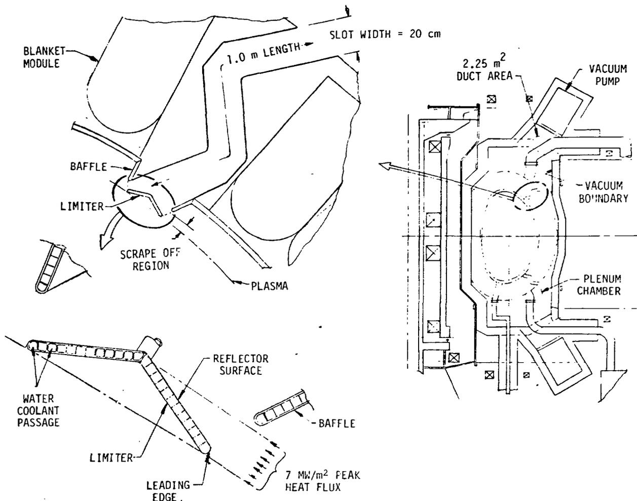
Figure 3. Limiter/vacuum duct concept.
