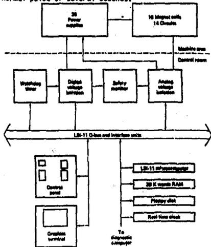
Fig. 2: Magnet Control System Block Diagram
