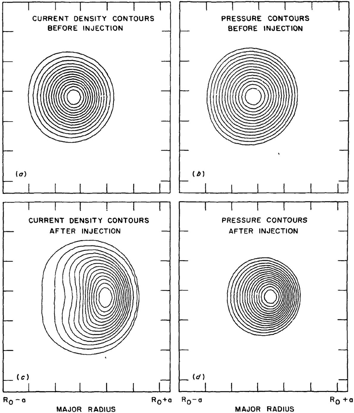
Fig. 4. The pressure and current density level contours before and after injection for the case described in Figs. 2-3. Although the pressure profiles are circular before and after injection, the strong  $BXVP/B^2$  contribution to the local current density at high  $\beta$  produces strongly distorted, noncircular current density profiles.
