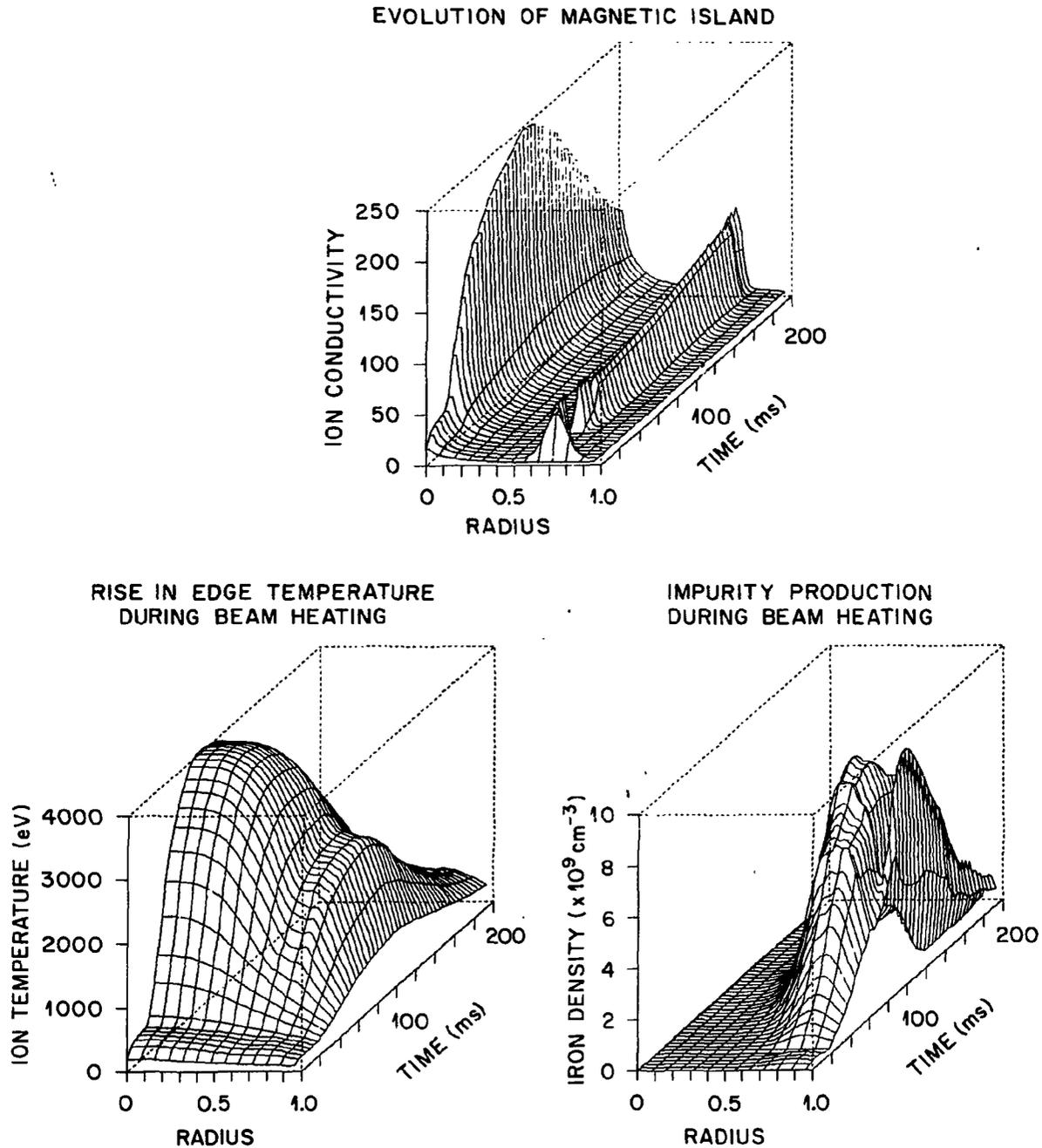
Fig. 10. The relationship between edge temperature, impurity production, impurity diffusion, and magnetic islands in an ISX-B neutral beam heating case. The rise in  $T_i$  edge due to heating leads to an increase in sputtered iron influx. The presence of a broad  $m = 2$  island retards the inward impurity flow.
