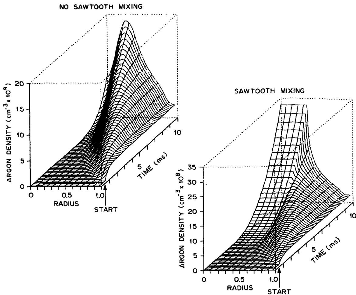
Fig. 9. Argon injection with/without sawtooth mixing. The uniform mixing of plasma parameters over the central zone leads to a quicker rise in the observed central radiation.
