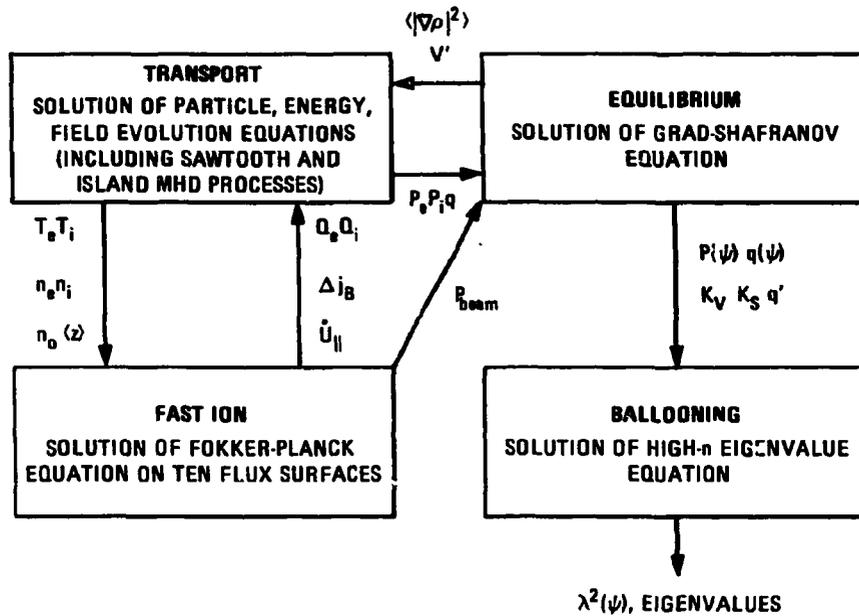
Fig. 1. Models used in ballooning-transport calculation. The radial Fokker-Planck transport processes (conduction, convection, beam heating, charge exchange, radiation) provide the pressure and shear profile for the 2-D equilibrium. The equilibrium variables determine the state of ballooning stability. When significant ballooning effects are discovered it may be possible to close the loop and to modify transport rates in regions of ballooning instability.
