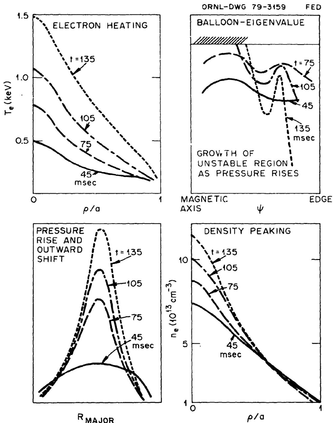
Fig. 3. Computer parameter evolution during ISX-B neutral beam heating (case shown in Fig. 2). The strong central peaking in pressure leads to a central zone of predicted ballooning instability (shaded region). The eigenvalues evolve from completely negative (stable) to mixed values as  $p'$  increases near the center.
