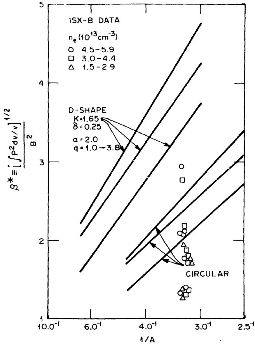
Fig. 5. Comparison of measured ISX-B  $\beta^*$  values with predicted critical  $\beta^*$  for circular plasma from the PEST code. Because possible noncircularity and pressure profile peaking are opposing, these values indicate the  $\beta^* > \beta^*_{\text{critical}}$  for these cases.
