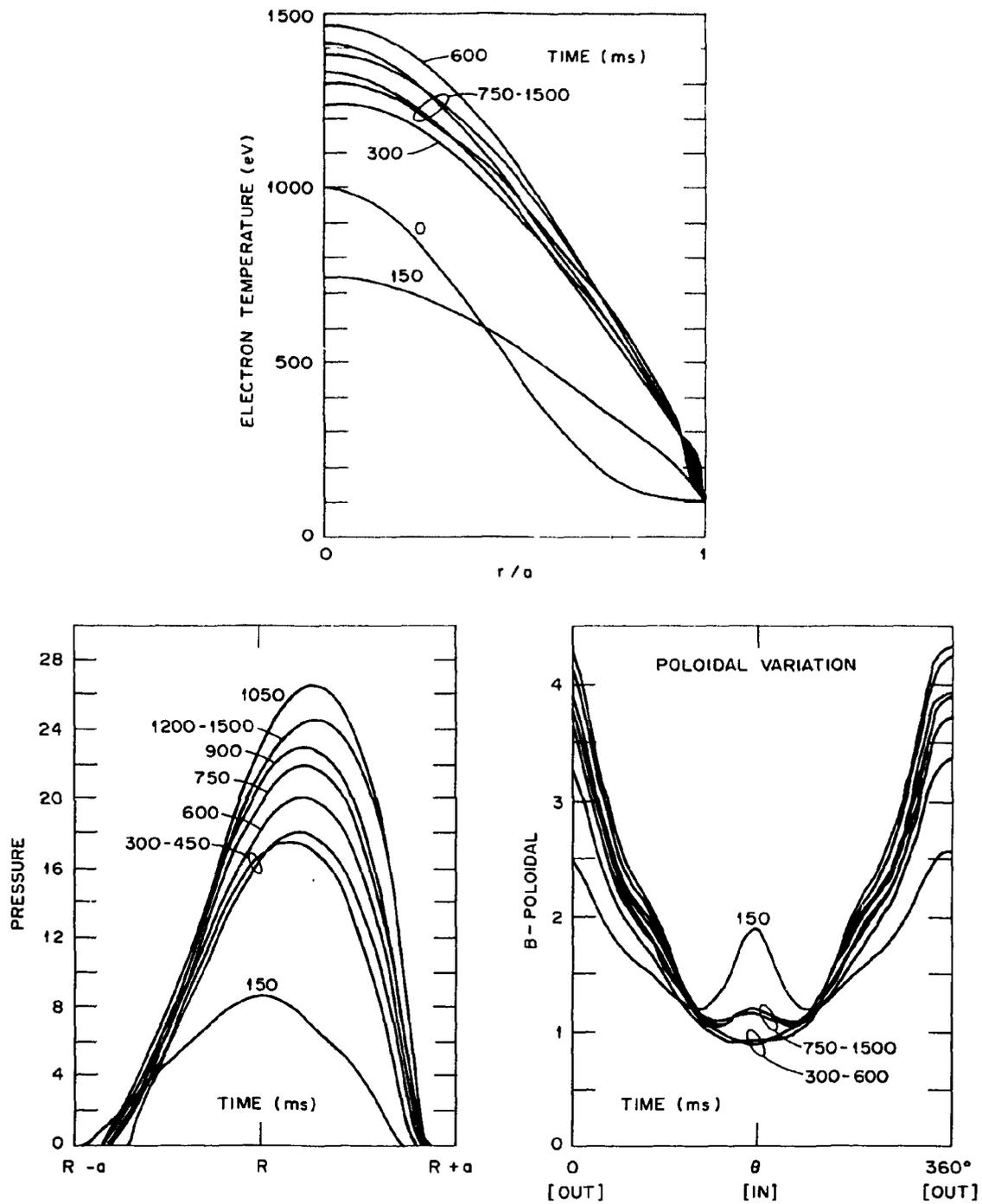
Fig. 11. Evolution of the ISX-B case considered earlier (Figs. 2-4) for 1.5 s. The poloidal field on the inside of the torus drops toward zero but reverses as impurities enter and  $\beta_{pol}$  decreases.
