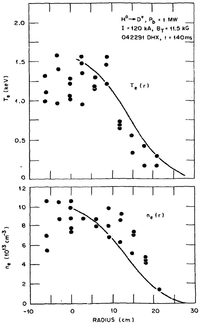
Fig. 2. Thomson scattering results for electron temperature and density profiles in an ISX-B 1-MW heating case. Although Alcator scaling and iron radiation combine to produce satisfactory agreement of code profiles with the data, the aim is simply to reproduce the thermal pressure profile for use in equilibrium and stability calculations.
