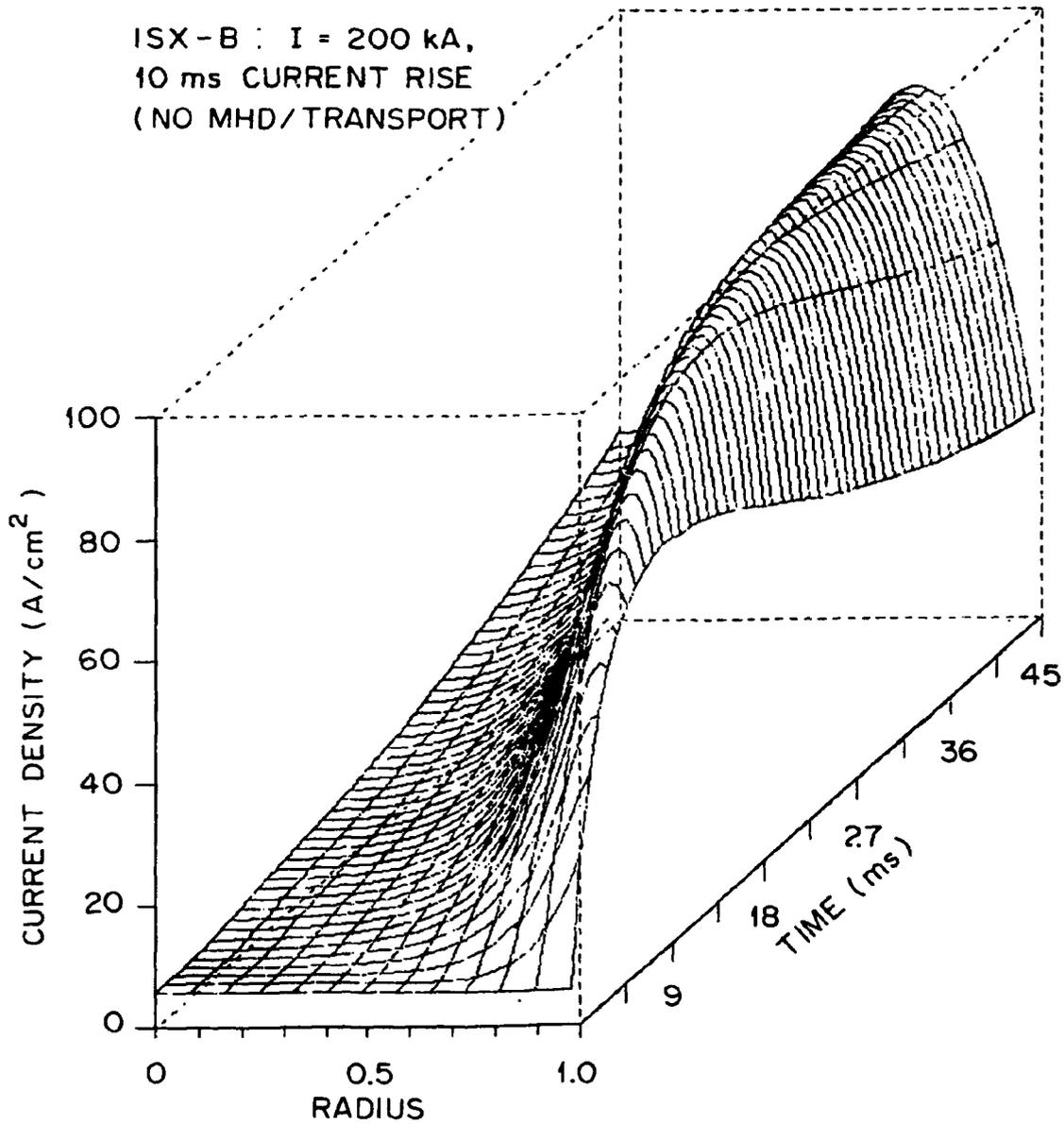
Fig. 6. Current penetration calculated for ISX-B without the MHD relaxation model. The attempt to produce a 200-kA current in 25 ms leads to a pronounced edge peaking of the current, unlike that of the experimental observation.
