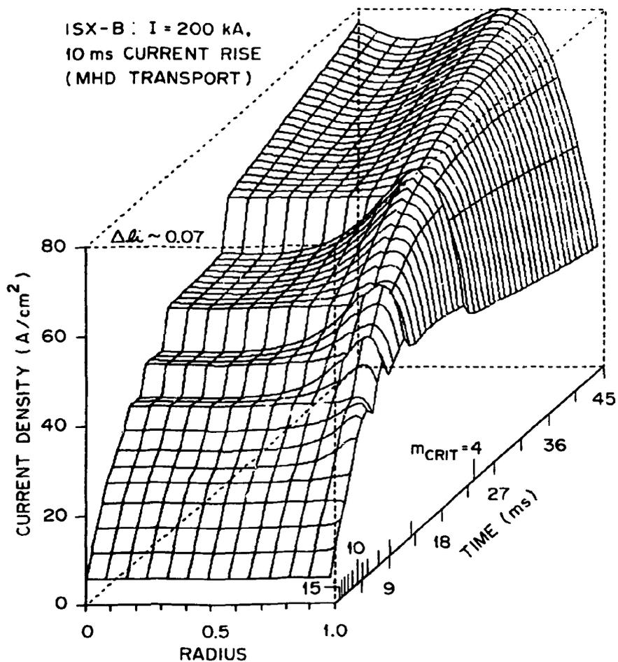
Fig. 7. Current penetration for the case of Fig. 6 with the MHD reconnection model. The periodic redistribution of flow gives an associated plasma shift (proportional to  $\Delta l_i$ ). This shift leads to the enhanced probability of arcing, with the high  $T_e$  plasma contacting the wall or limiter.
