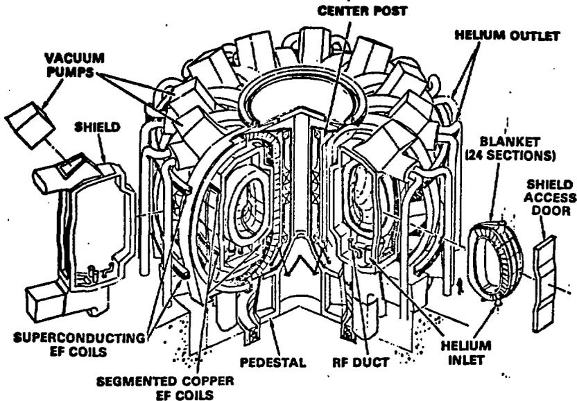
Figure 1. Starfire Reactor Design
