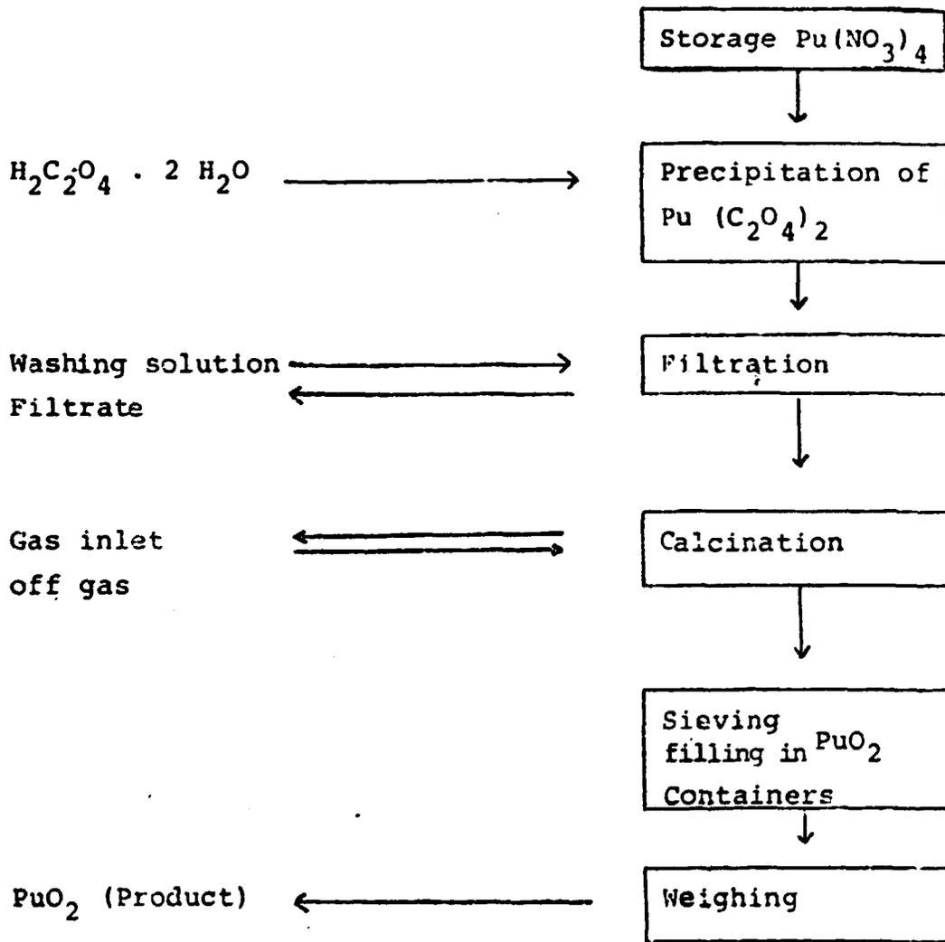
Fig. 1 Conversion flow sheet
