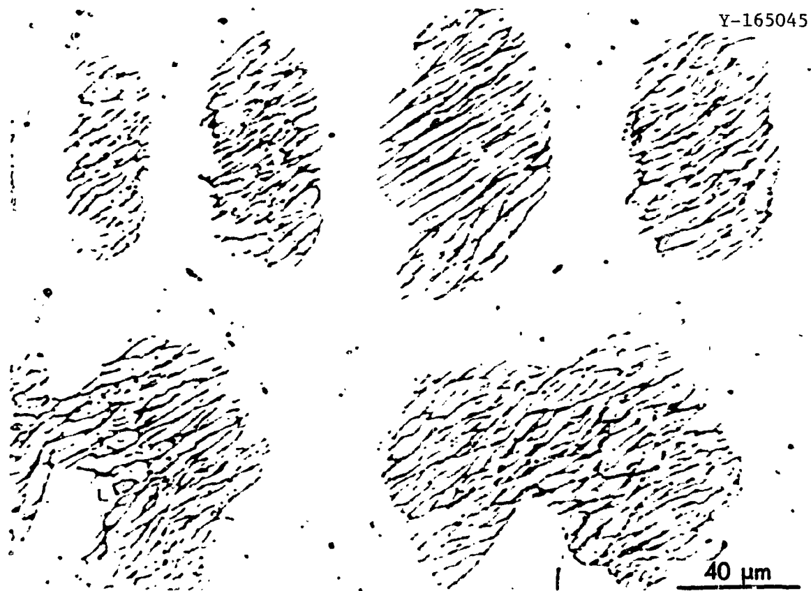
Fig. 4. Interrupted Solidification Sample Quenched from 1365°C.
