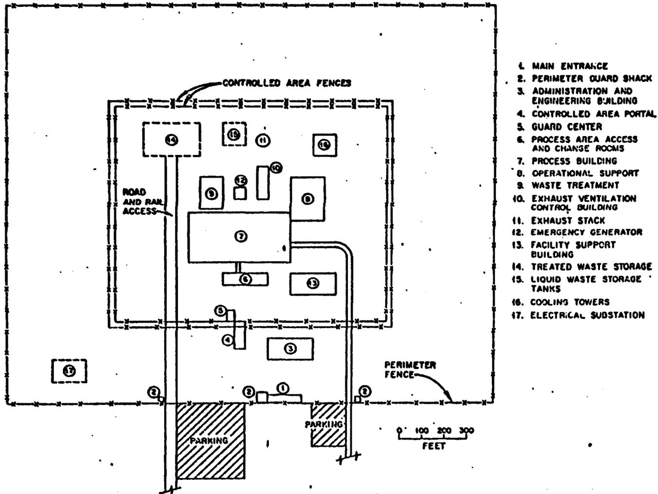
Fig. 4.1 Site Plan for a 200-MTHM/yr Sphere-Pac LWR Fabrication Plant.
