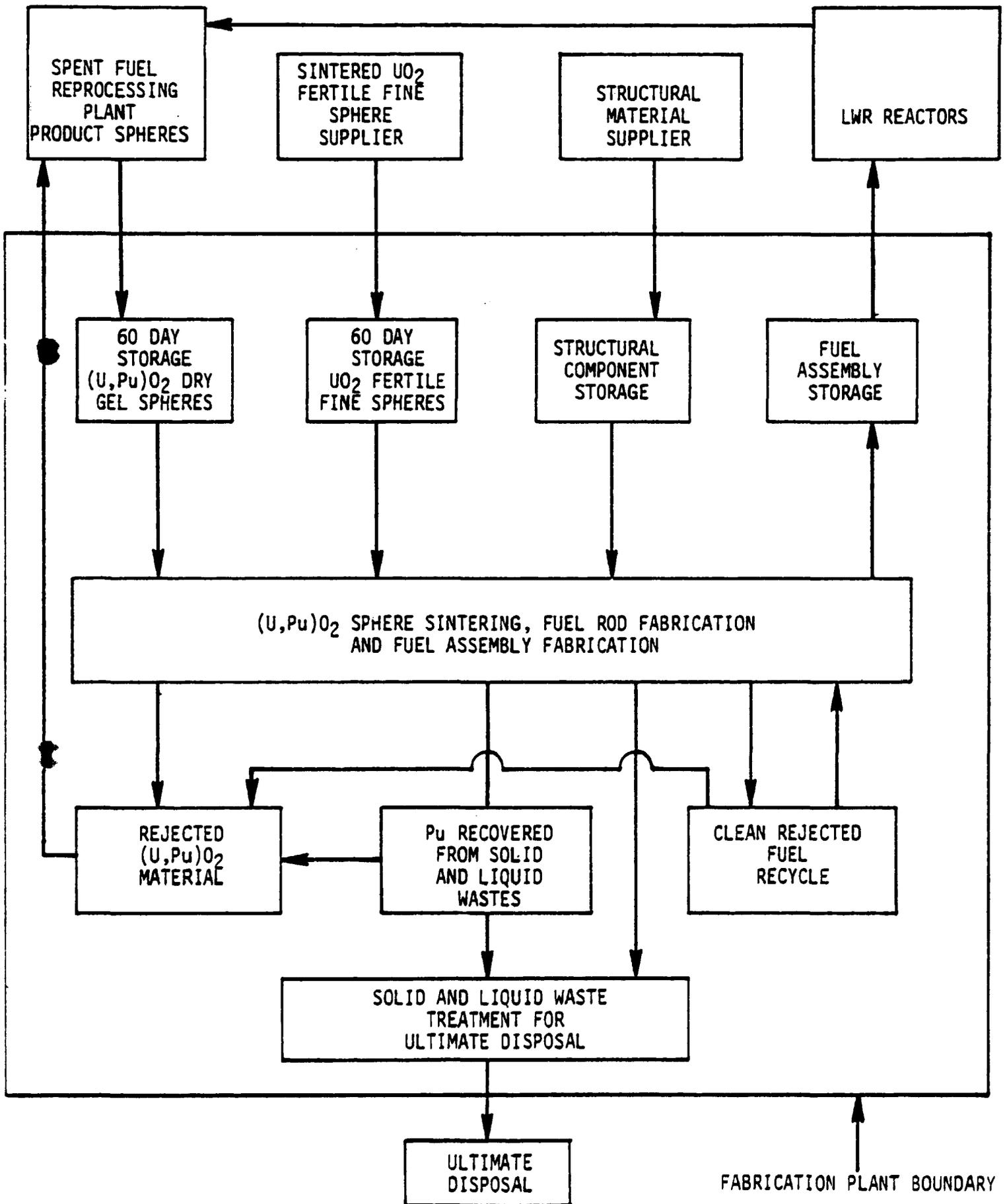
Fig. 2.1. LWR Recycle Pu Fuel Fabrication Plant.
