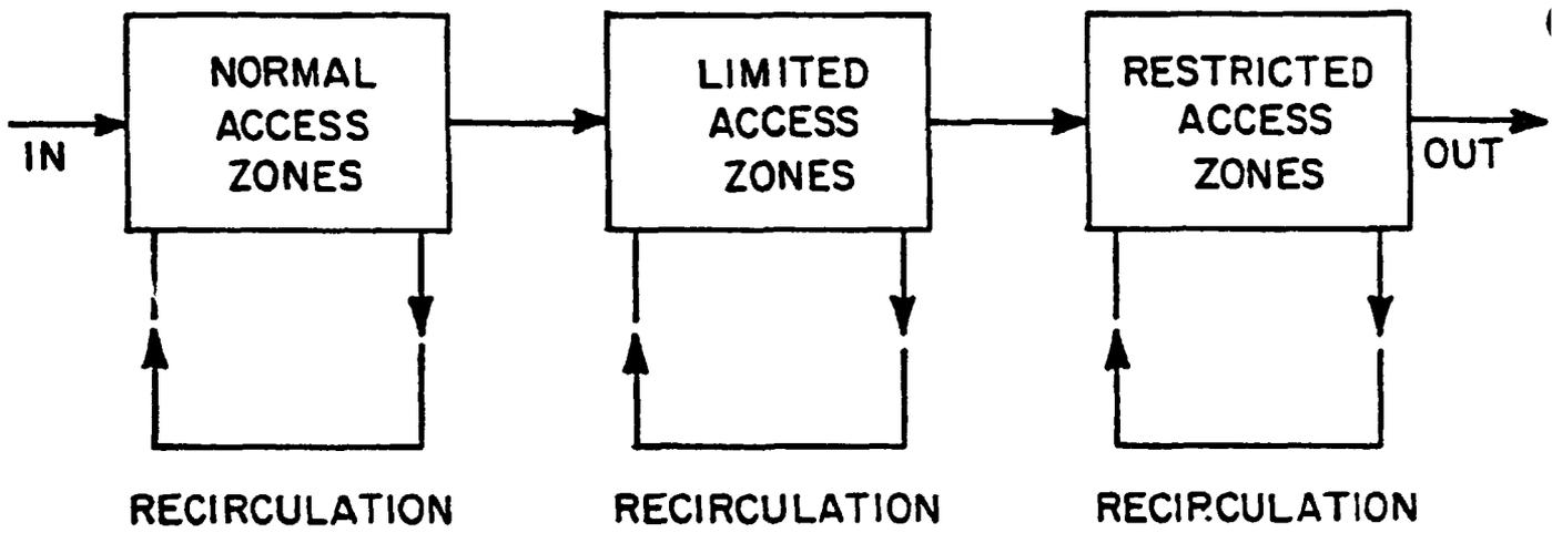
Fig. 5.1 Schematic Diagram of Fuel Fabrication Building Airflow.
