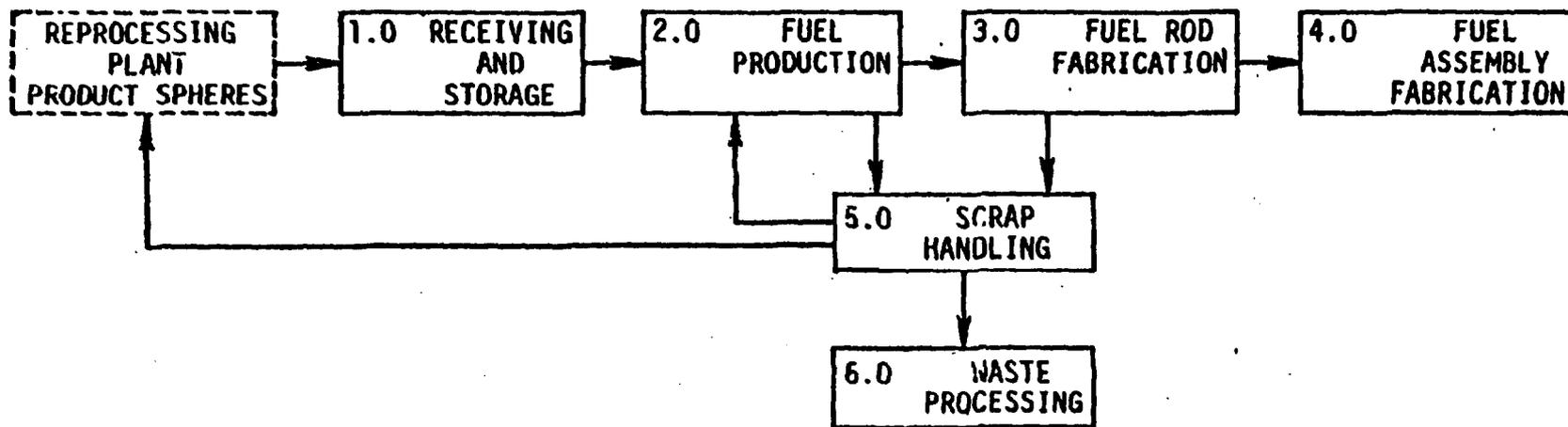
Fig. 3.1 Gel-Sphere-Pac Generic Fuel Refabrication Functional Flowsheet,
