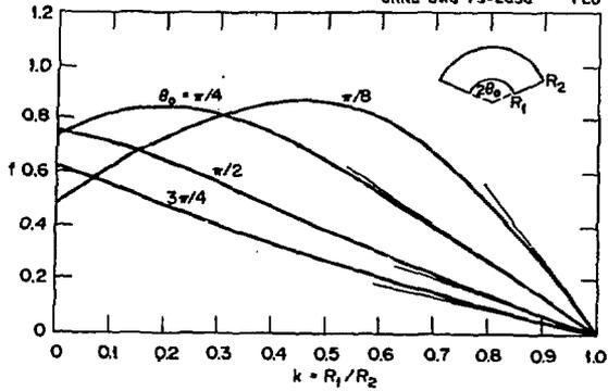
Fig. 3. Sikora's curves of  $f$  for sectors of circular annuli together with the exact slopes at  $k = 1$ .
