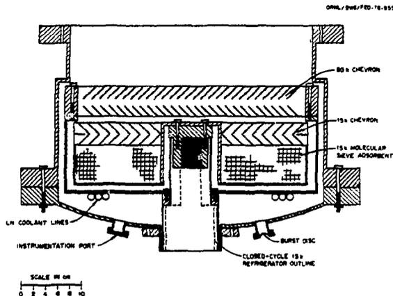
Figure 2. Cross section of INS cryosorption pump.
