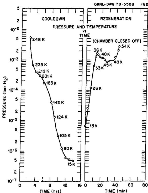
Figure 3. Cooldown and regeneration-pressure and temperature vs time.
