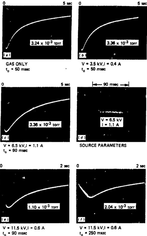
Figure 4. (a), (b), (c), (e), and (f): Pressure vs time for various ion source parameters. Labels give peak pressure during pulse. (d): Source parameters for plot (c).  $t_0$  = beam pulse length.
