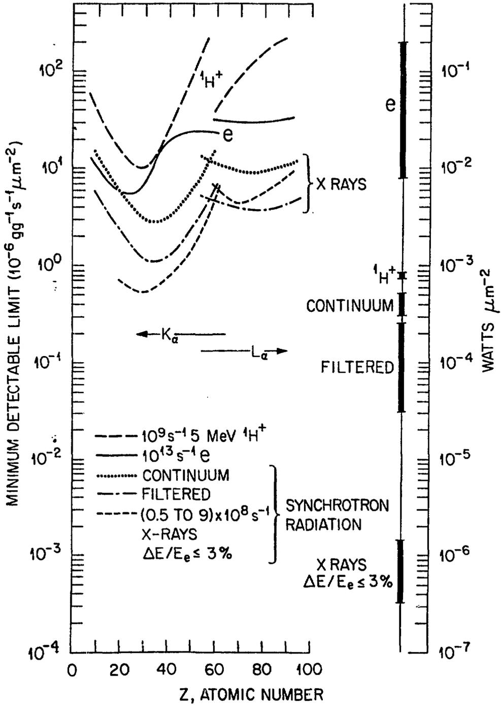
Figure 1. Comparisons of minimum detectable limits for thick samples and power dissipated among charged-particle and synchrotron radiation fluorescence microprobes (after Sparks (3)).
