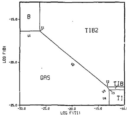
Fig. 1. Stability diagram for condensed Ti-B phases at 1200K.
