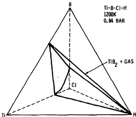
Fig. 4. TiB<sub>2</sub> + Gas phase field at 1200K.
