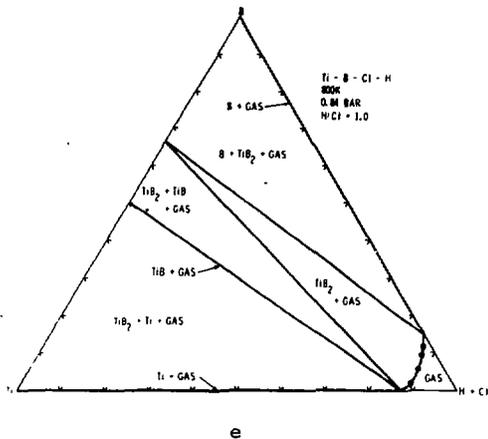
TiB<sub>2</sub> + Gas field is the main phase field of interest since TiB<sub>2</sub> is the desired condensed phase and a schematic three dimensional view of this field at 1200K is shown in Figure 4. On the Ti-B-Cl face, it is roughly
