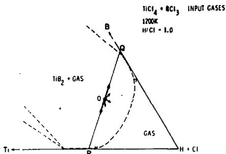
Fig. 9. Superposition of the phase diagram and accessibility diagram for  $\text{TiCl}_4$  and  $\text{BCl}_3$  source gases at 1200K,  $\text{H/Cl} = 1$ .
