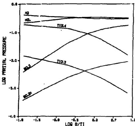
Fig. 5. Calculated partial pressures of major gas species along the 1200K  $TiB_2$  + Gas/Gas boundary for  $H/Cl = 1$  ( $U_2$  in Figure 3b).
