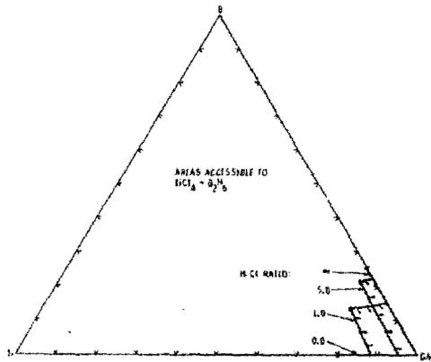
Fig. 11. Accessible areas of the Ti-B-Cl-H system for  $\text{TiCl}_4$  and  $\text{B}_2\text{H}_6$  source gases at  $\text{H}/\text{Cl} = 0, 1, 5, \infty$ .
