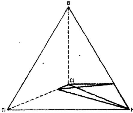
Fig. 10. Accessible volume of the Ti-B-Cl-H system for  $\text{TiCl}_4$  and  $\text{B}_2\text{H}_6$  source gases.
