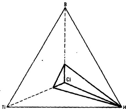
Fig. 7. Accessible volume of the Ti-B-Cl-H system for  $\text{TiCl}_4$  and  $\text{BCl}_3$  source gases.
