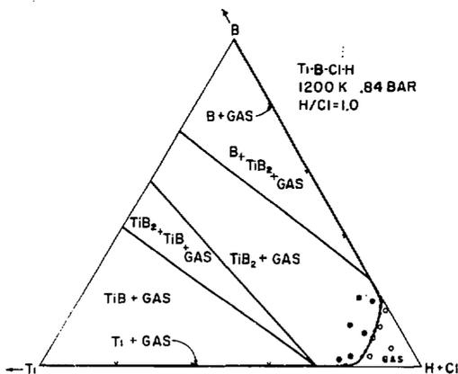
Fig. 6. Experimental verification of the calculated  $TiB_2 + Gas/Gas$  boundary ( $U_2$ ). Large filled circles represent CVD conditions where  $TiB_2$  deposits were observed, unfilled circles represent conditions where no deposits were observed. Smaller dots correspond to calculated points along  $U_2$  in Figure 3b.
