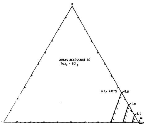
Fig. 8. Accessible areas of the Ti-B-Cl-H system for  $\text{TiCl}_4$  and  $\text{BCl}_3$  sources gases at  $\text{H/Cl} = 0, 1, 5, \infty$ .
