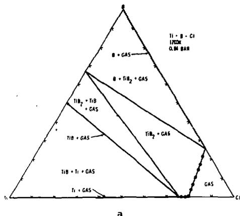
Fig. 3. Calculated Ti-B-Cl-H phase diagrams at 0.84 bar total pressure. a) 1200K, H/Cl = 0, b) 1200K, H/Cl = 1, c) 1200 and 800K, H/Cl = ∞, d) 800K, H/Cl = 0, e) 800K, H/Cl = 1. Axes are marked at 10% intervals. Filled circles indicate calculated points on U2.
