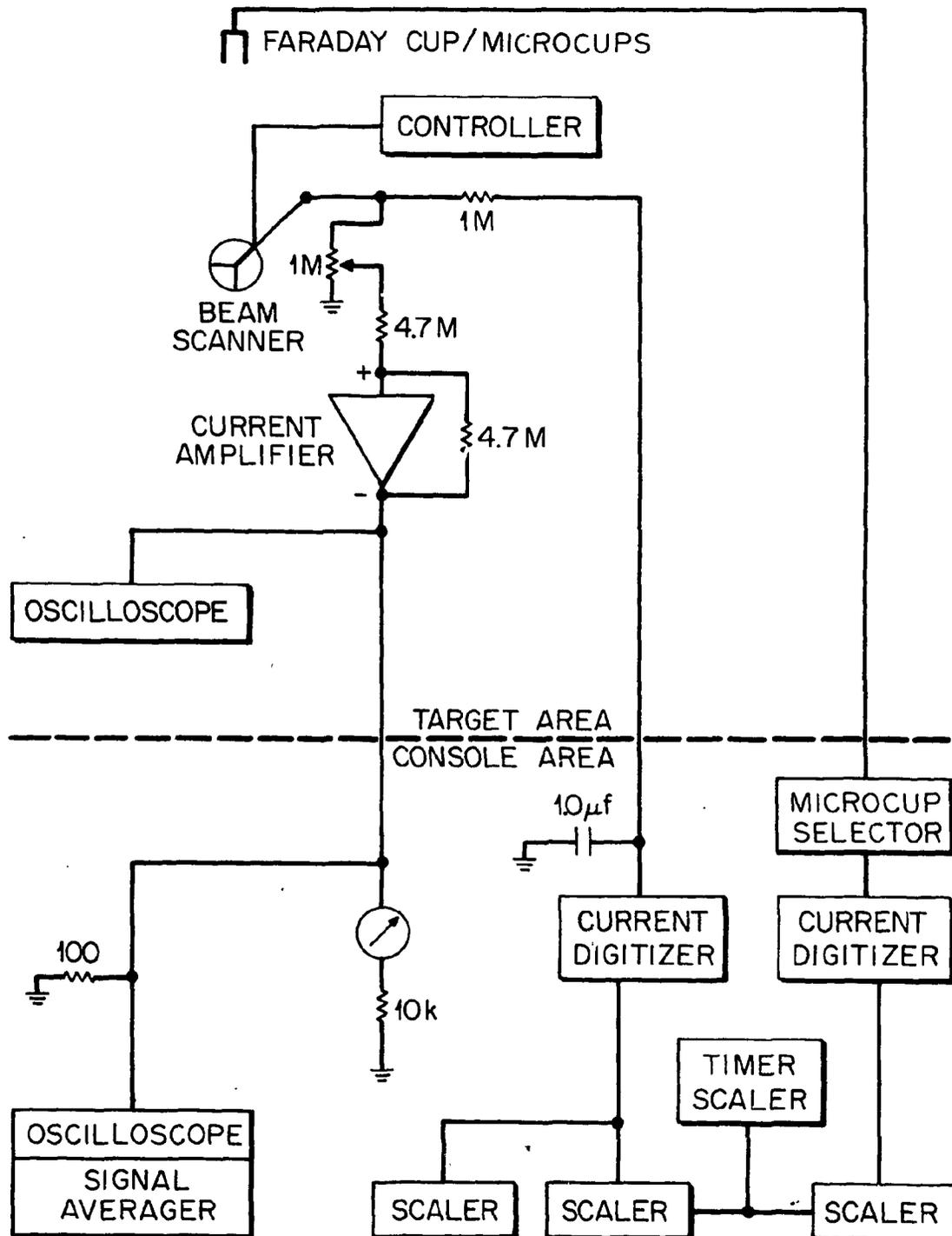
Fig. 7. Block Diagram of Electronics for the Beam Monitoring System. Signals originate at the beam scanner (continuously in service) or at the Faraday cup or microcups used at selected times. The current signals are then routed to measurement devices located at the Van de Graaff console area.
