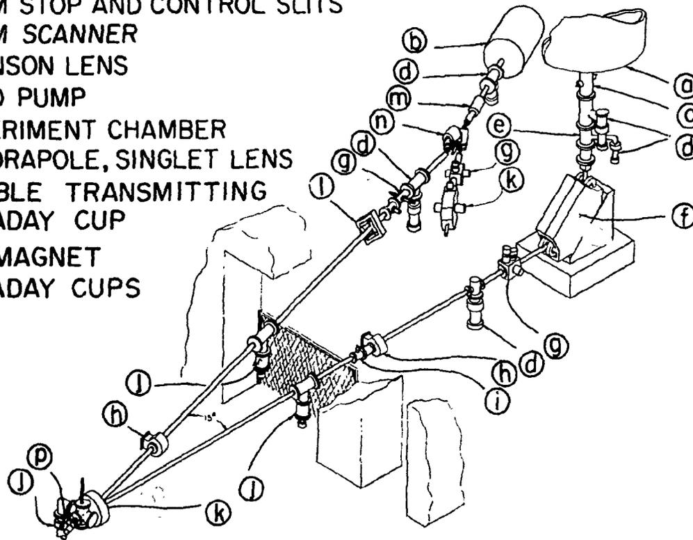
Fig. 1. Schematic of the Two Accelerators and Their Respective Beam Lines to the Radiation Damage Target Chamber (Lower Left).
