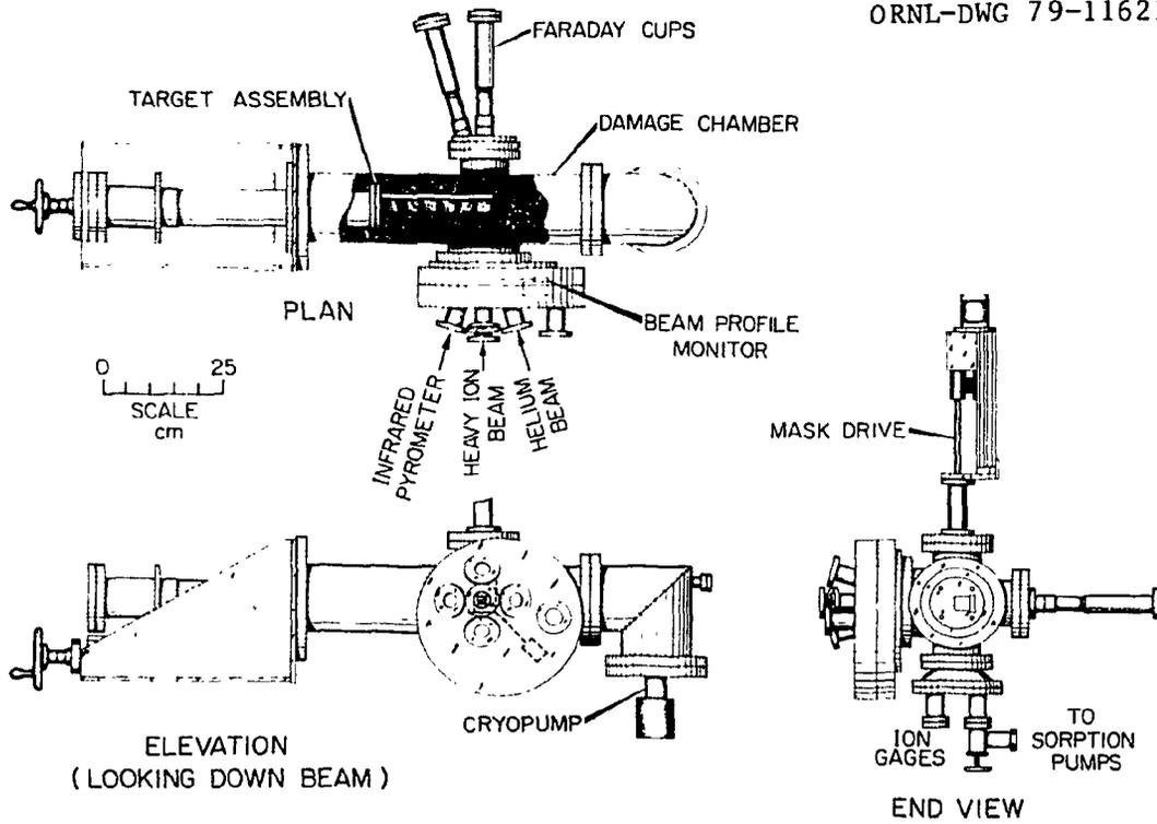
Fig. 2. Layout of the Radiation Damage Target Chamber.
