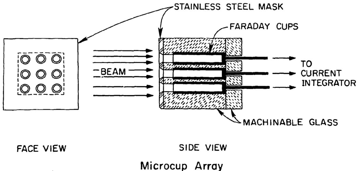
Fig. 8. Two Schematic Views of the Nine-Hole Miniature Faraday Cup Array Used to Assess the True Beam Intensity on Each Target Disk.
