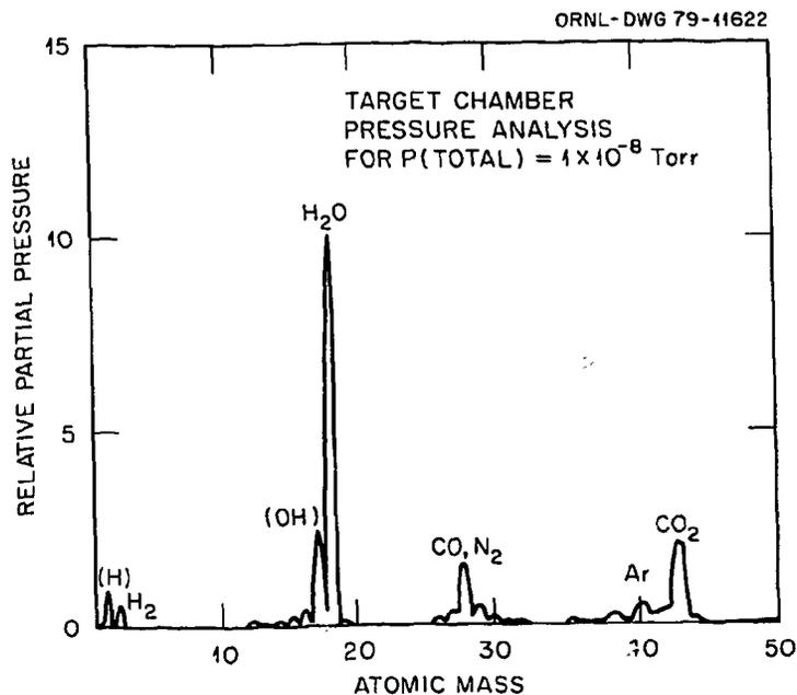
Fig. 4. Residual Gas Analyzer Spectrum of Target Chamber Atmosphere. Pressure:  $1 \times 10^{-8}$  torr =  $1.3 \times 10^{-6}$  Pa.
