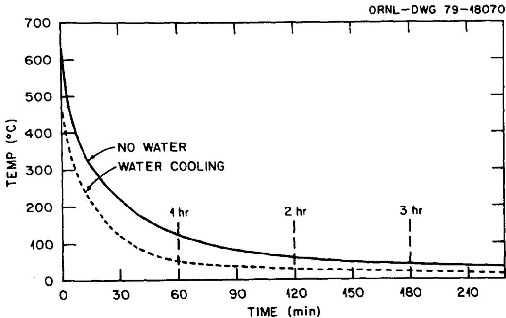
Fig. 3A. Time Required for a Specimen in Station 1 at the End of the Target Assembly to Cool from 700°C Either With or Without the Use of Cooling Water. Holding time at 700°C before cooldown was 75 min.
