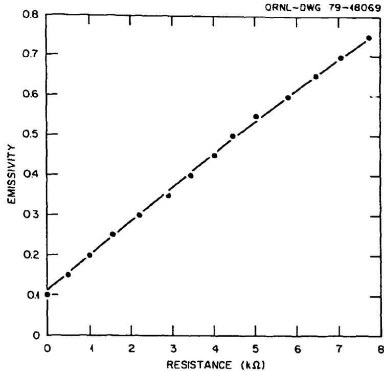
Fig. 2A. Calibration Curve for the Raytek SL 300 SC Infrared Pyrometer, Relating Resistance Value of the ORNL-Installed Ten-Turn Potentiometer to the Original Factory-Calibrated Emissivity Function.
