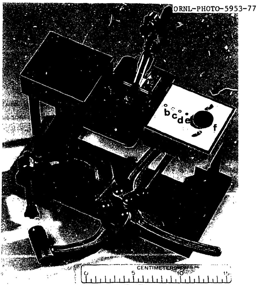
Fig. 6. Disassembled Specimen Holder in the Loading Jig. Components are: (a) face plate, (b) miniature bar mask, (c) platinum wire gasket, (d) optional 0.05-mm-thick oxidized stainless steel spacer, (e) specimen, and (f) thermalizer block.
