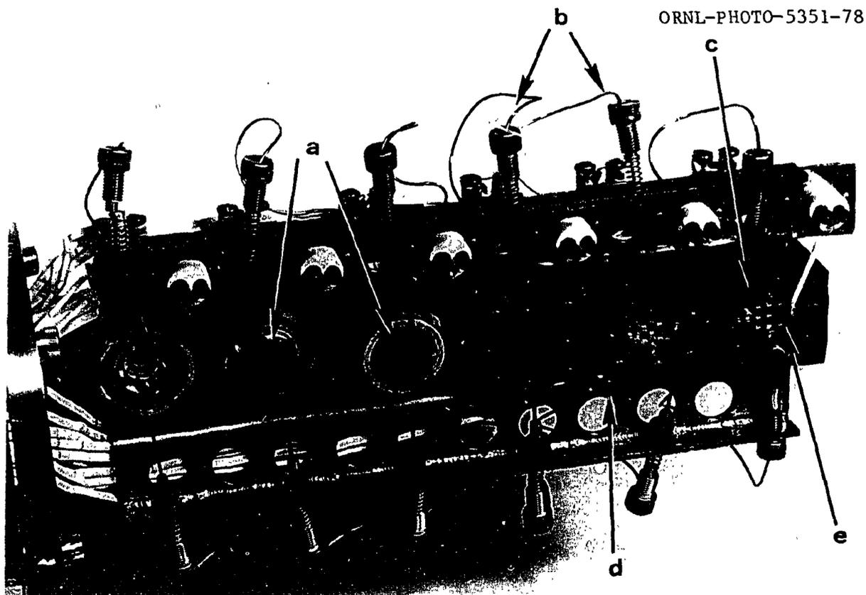
Fig. 5. Detailed View of the Target Assembly Showing the Six Heater Stations in Progressive Stages of Assembly from Left to-Right, including: (a) Electron Guns, (b) Spring-Loaded Thermalizer Block Thermocouples, (c) Nine-Disk Specimen Holder, (d) Tantalum Heat Shield, and (e) Specimen Thermocouple.
