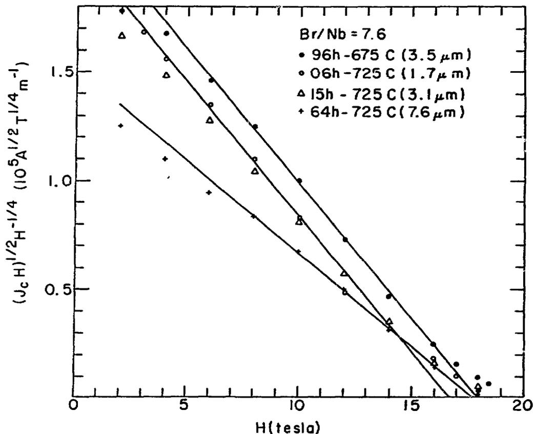
Fig. 6. Plots for  $J_c^{1/2} H^{1/4}$  vs  $H$  for a series of  $Nb_3Sn$  wires which were heat treated for 6, 16, and 64 h at  $725^\circ C$  and for 96 h at  $675^\circ C$ .
