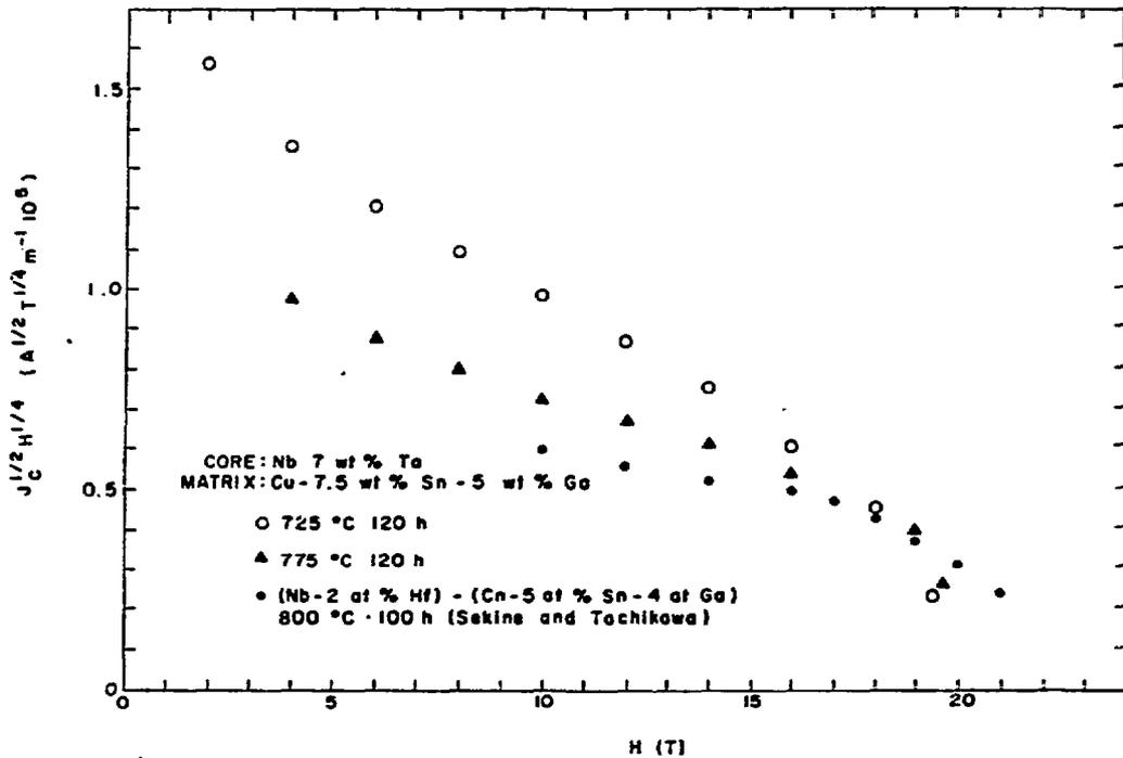
Fig. 4.  $J_C^{1/2} H^{1/4}$  vs H for Ga-containing  $Nb_3Sn$  wires. These data do not appear to obey Eq. (2).
