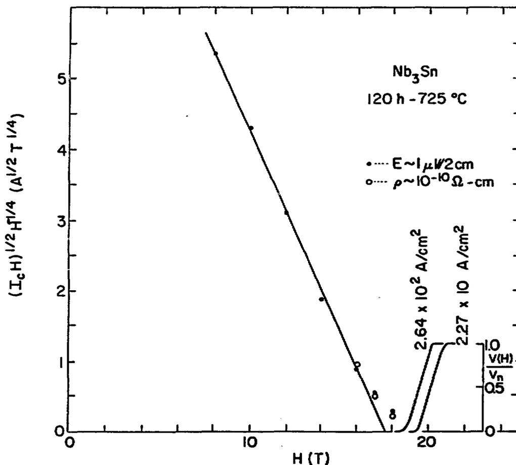
Fig. 1. A plot for  $J_c^{1/2} H^{1/4}$  vs  $H$  for a monofilamentary  $\text{Nb}_3\text{Sn}$  wire which was heat treated at  $725^\circ\text{C}$  for 120 h indicating the extrapolated  $H_{c2}$  and the low current density  $H_{c2}$ .
