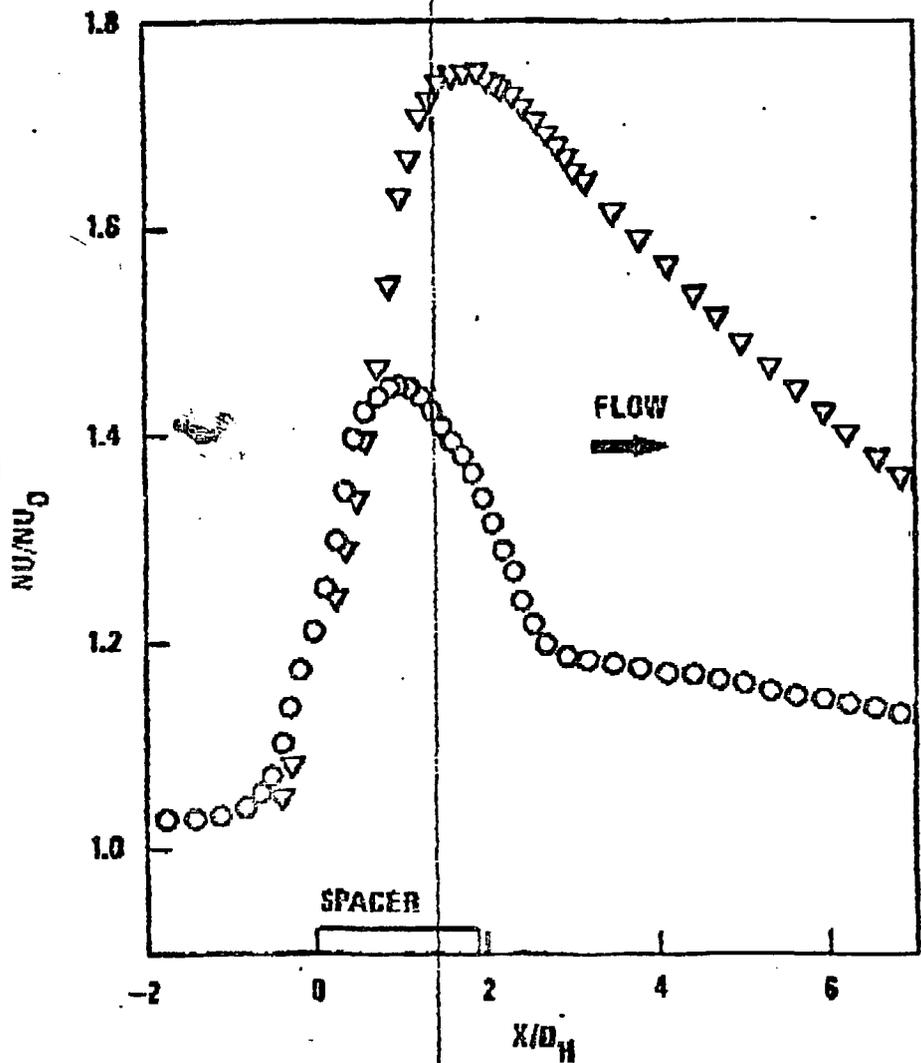
Fig. 6. Axial distribution of the Nusselt numbers measured between the ribs of the spacers  $\nabla$  smooth;  $\circ$  rough (Ref. 39).
