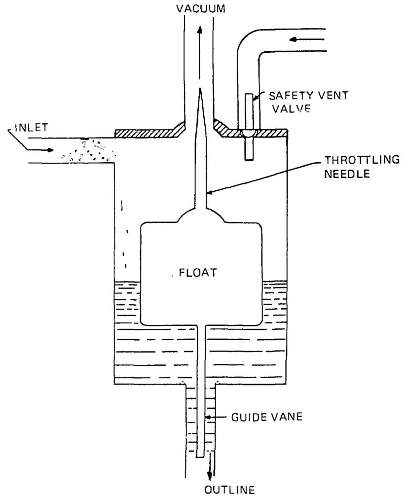
FIGURE 2: AIR SEPARATOR POT
